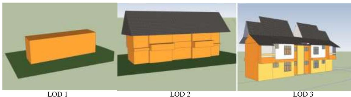
**Figure 9.** Resulted model in LOD 1, LOD 2, and LOD 3.
