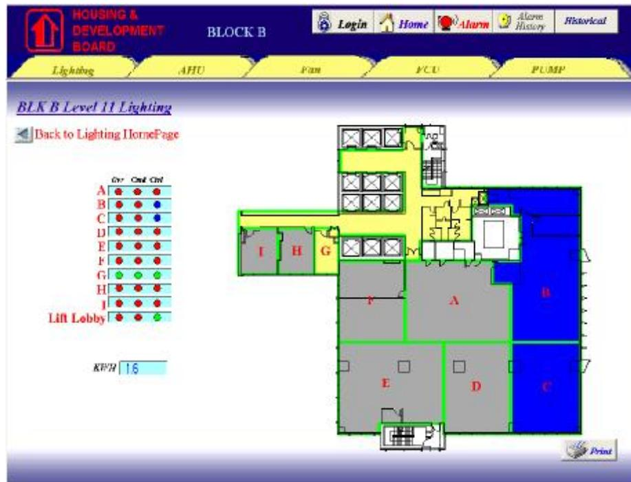
**Figure 4.3 iFix Intellution SCADA View for Lighting**
