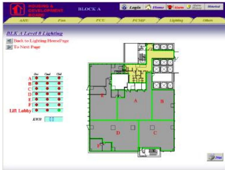
Figure 5.13 SCADA Display For Light Zonings
