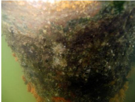
Fig. 1. Photo of Barnacles growth at hull boat<sup>1</sup>
