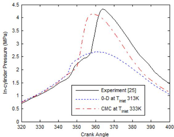
**Figure 4** Combustion behaviours when the intake temperature was changed for both models.
