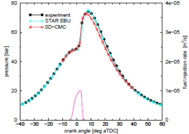
Figure 3 0-D CMC and a multi-dimensional simulation (STAR EBU) compared with experiment [14]
