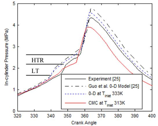
Figure 2 Comparison of the in-cylinder pressure between experiment [25], 0-D from Guo et al. [25], 0-D in this study and CMC with 0-D.
