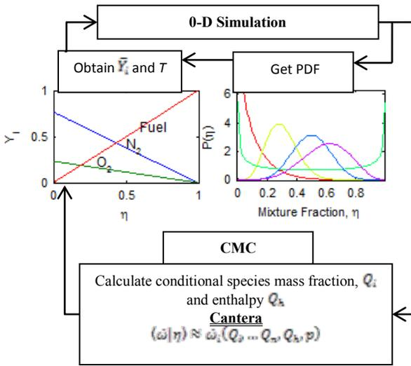
Figure 1 Interfacing between 0-D and CMC models.
