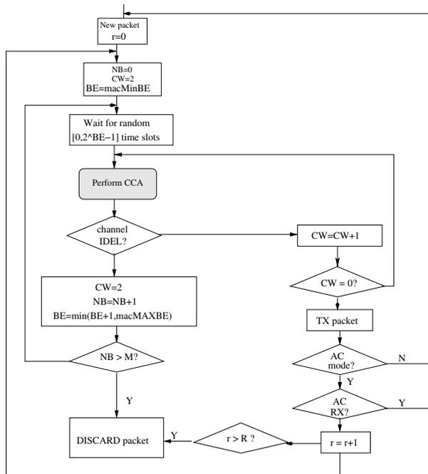
Fig. 3. Procedure of channel access with retransmission
