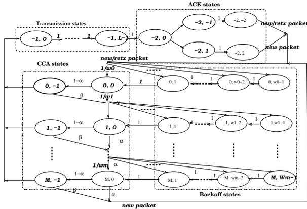
Fig. 4. Markov model for slotted CSMA/CA per node
