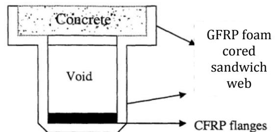
Figure 7. Hybrid box beam concept [18].
