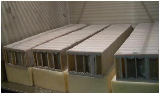
Figure 5. S-FRP sandwich bridge beam [14].
