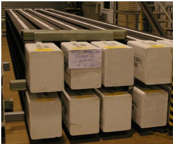
Figure 9. Glue-laminated sandwich bridge girder.
