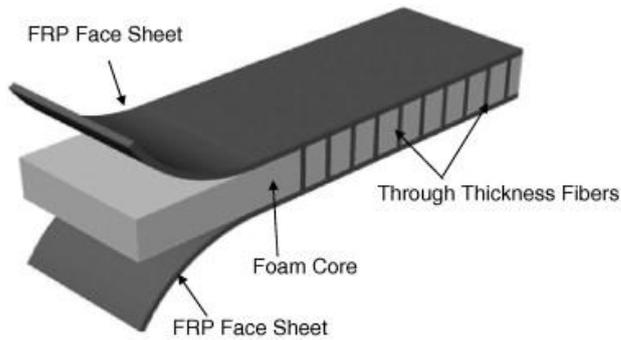
Figure 1. 3-D FRP sandwich panels [9].
