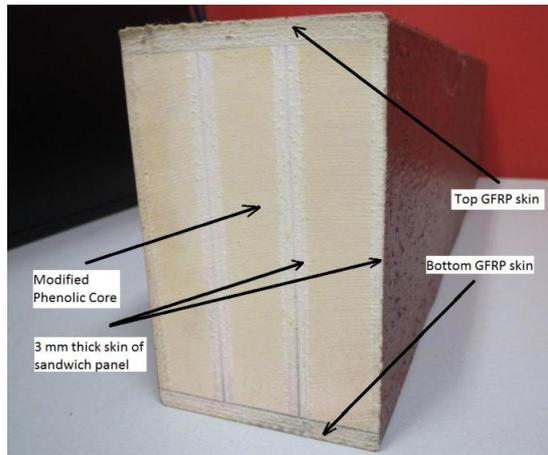
**Figure 15. Hybrid glulam composite sandwich beam**
