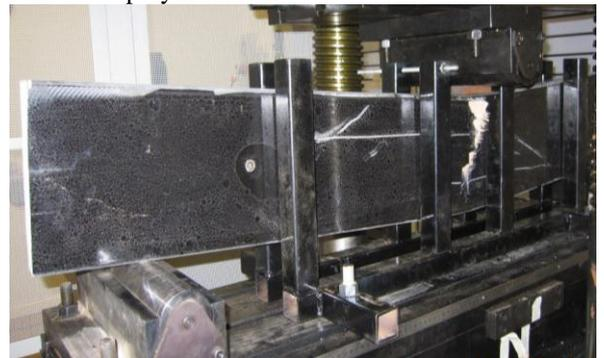
Figure 14. Flexural test of a sandwich waler
