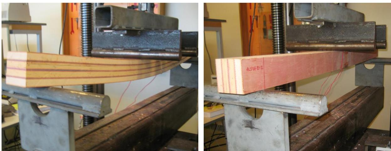
**Figure 2: Static bending test of glue-laminated sandwich beam.**
