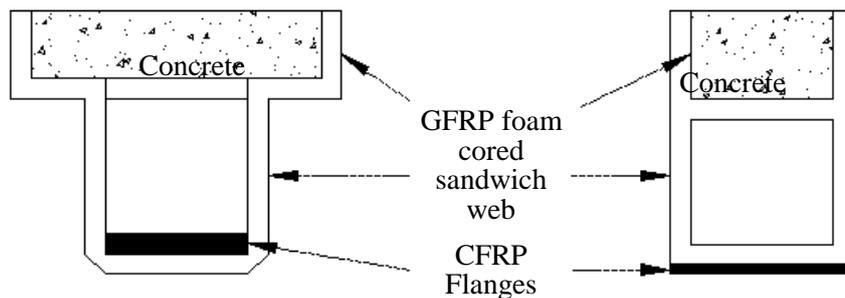
**Figure 1: Hybrid box beam concept (Canning et al. 1999).**
