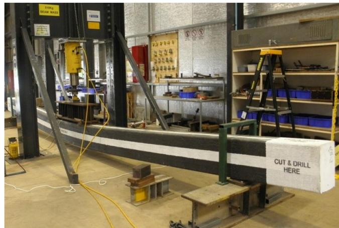
**Figure 6: Glue-laminated fibre composite sandwich bridge girder.**
