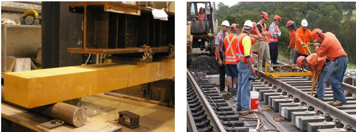
**Figure 3: Glue-laminated fibre composite sandwich railway sleepers.**
