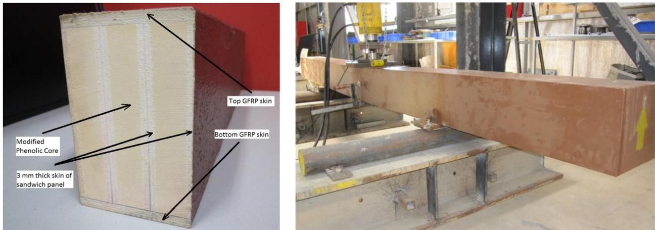
**Figure 7: Hybrid glue-laminated fibre composite sandwich beam.**
