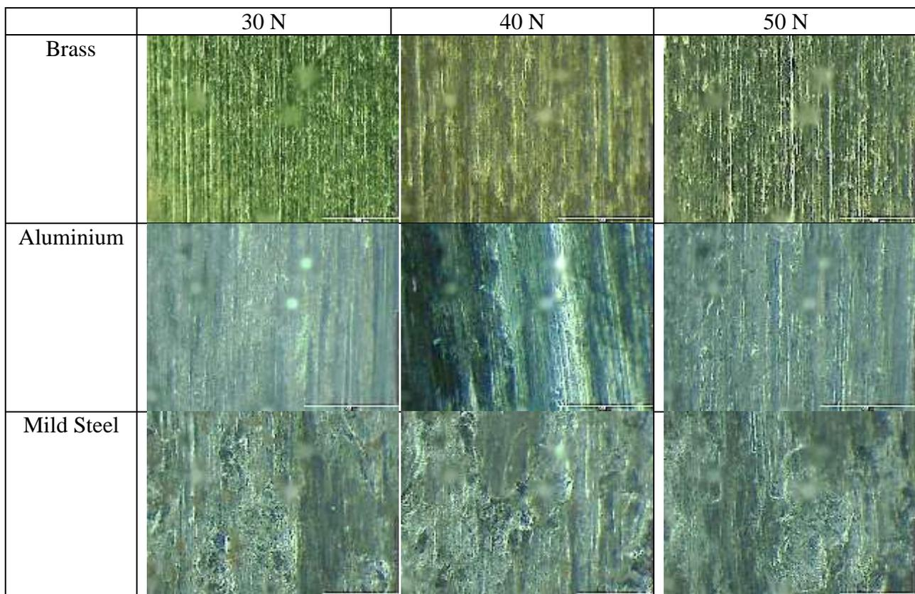
**Fig. 5** Micrographs of worn surface Roughness after the test at different applied loads after 10.9 km sliding distance.
