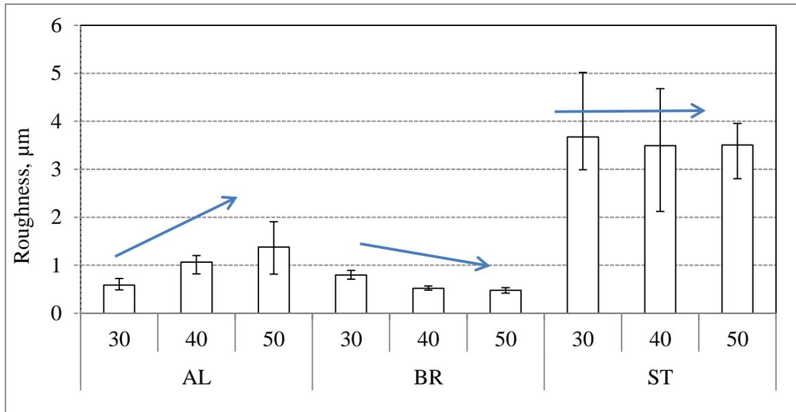
**Fig. 4** Average of worn surface roughness after the test at different applied loads after 10.9 km sliding distance.
