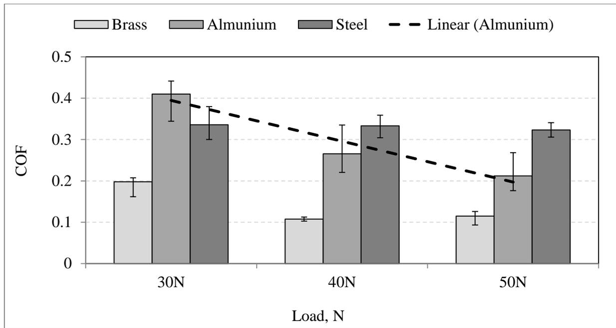
**Fig. 3** Summary of friction coefficient at steady state of brass, aluminium, mild steel materials under dry contact conditions at different applied loads after 10.9 km sliding distance.
