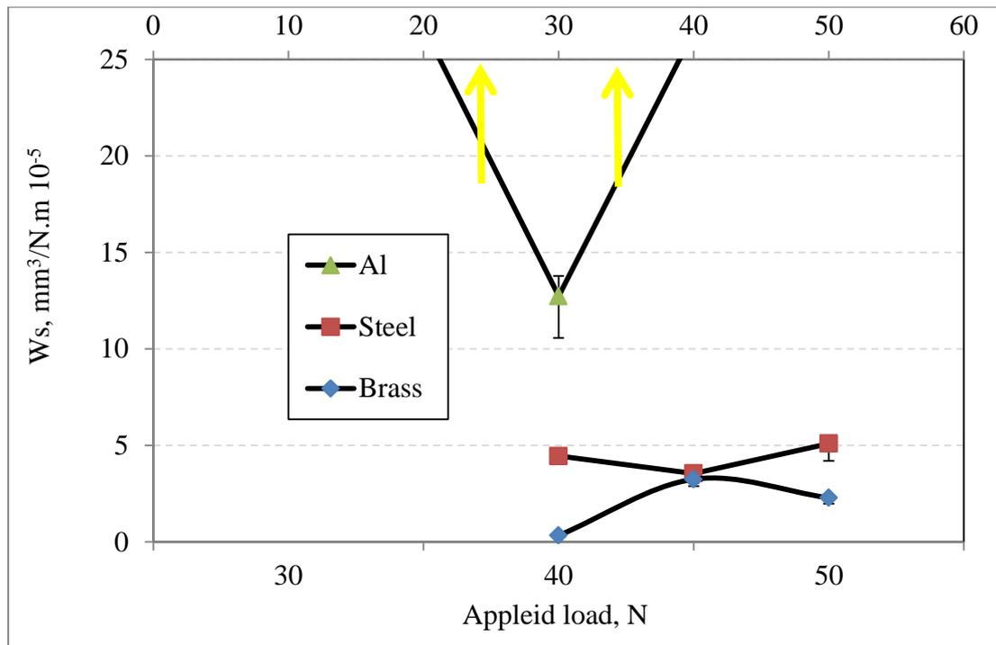
**Fig. 2** Summary of specific wear rate at steady state of brass, aluminium, mild steel materials under dry contact conditions at different applied loads after 10.9 km sliding distance.
