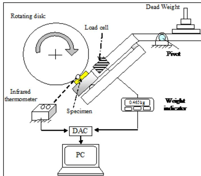
**Fig.1** configuration of block on ring machine
