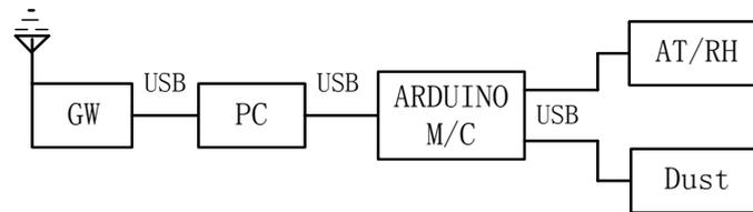
Fig.2 The vehicle measurement system structure
