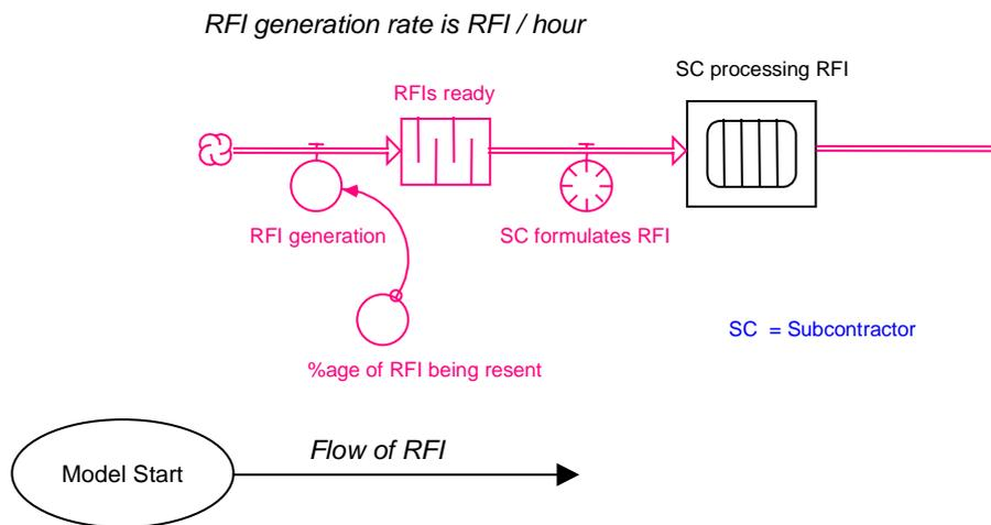
*Figure 5: Simulation diagram of RFI generation*
