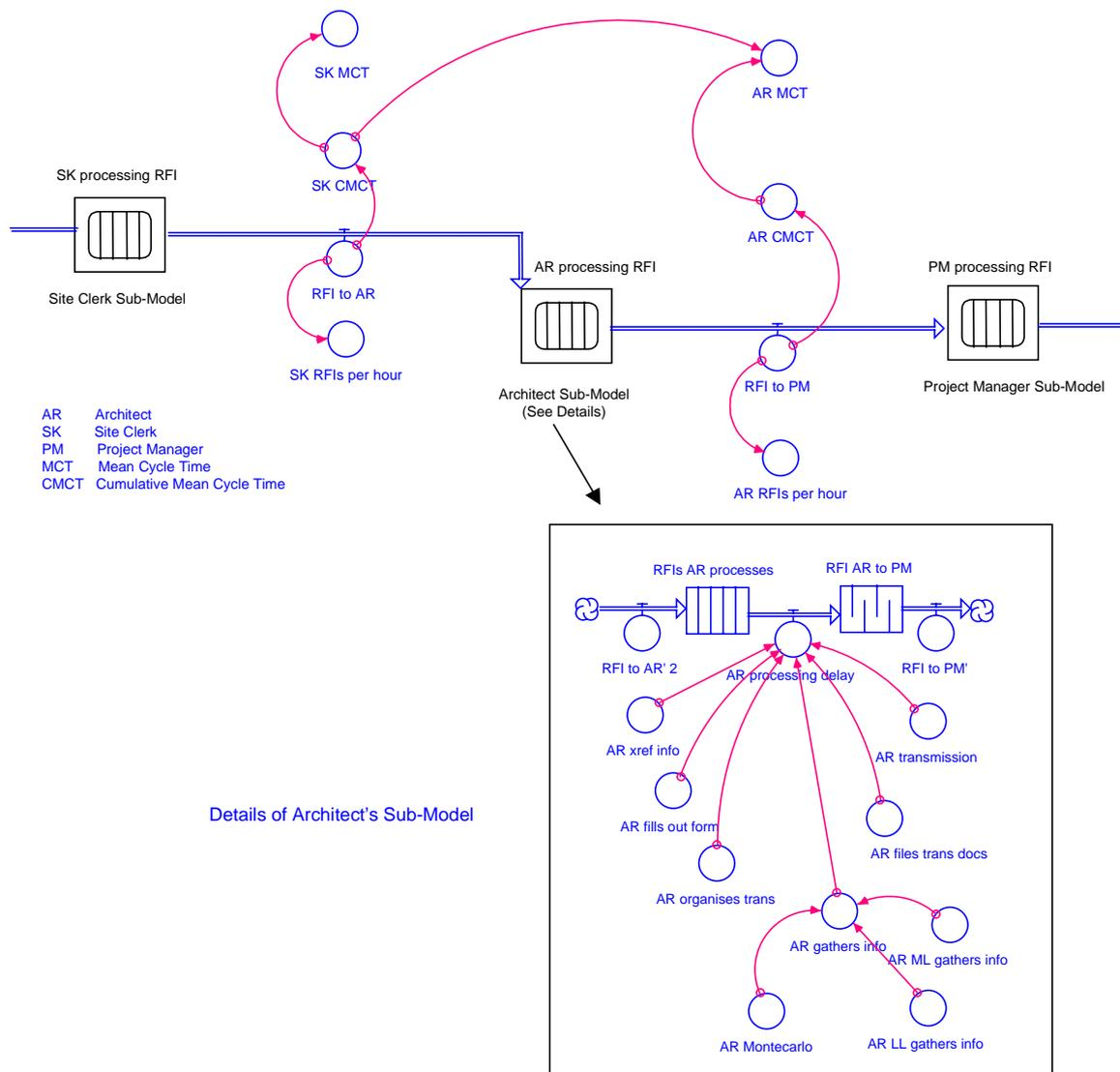
Figure 4: Part of the simulation model showing details of the Architect's sub-model
