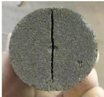
**Figure 2. Sample tested for tension.**
