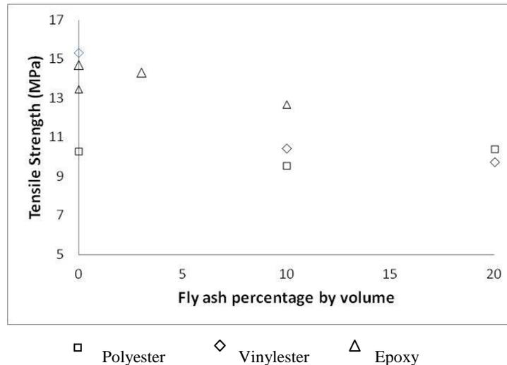
Figure 5. Variation of tensile strength with fly ash.
