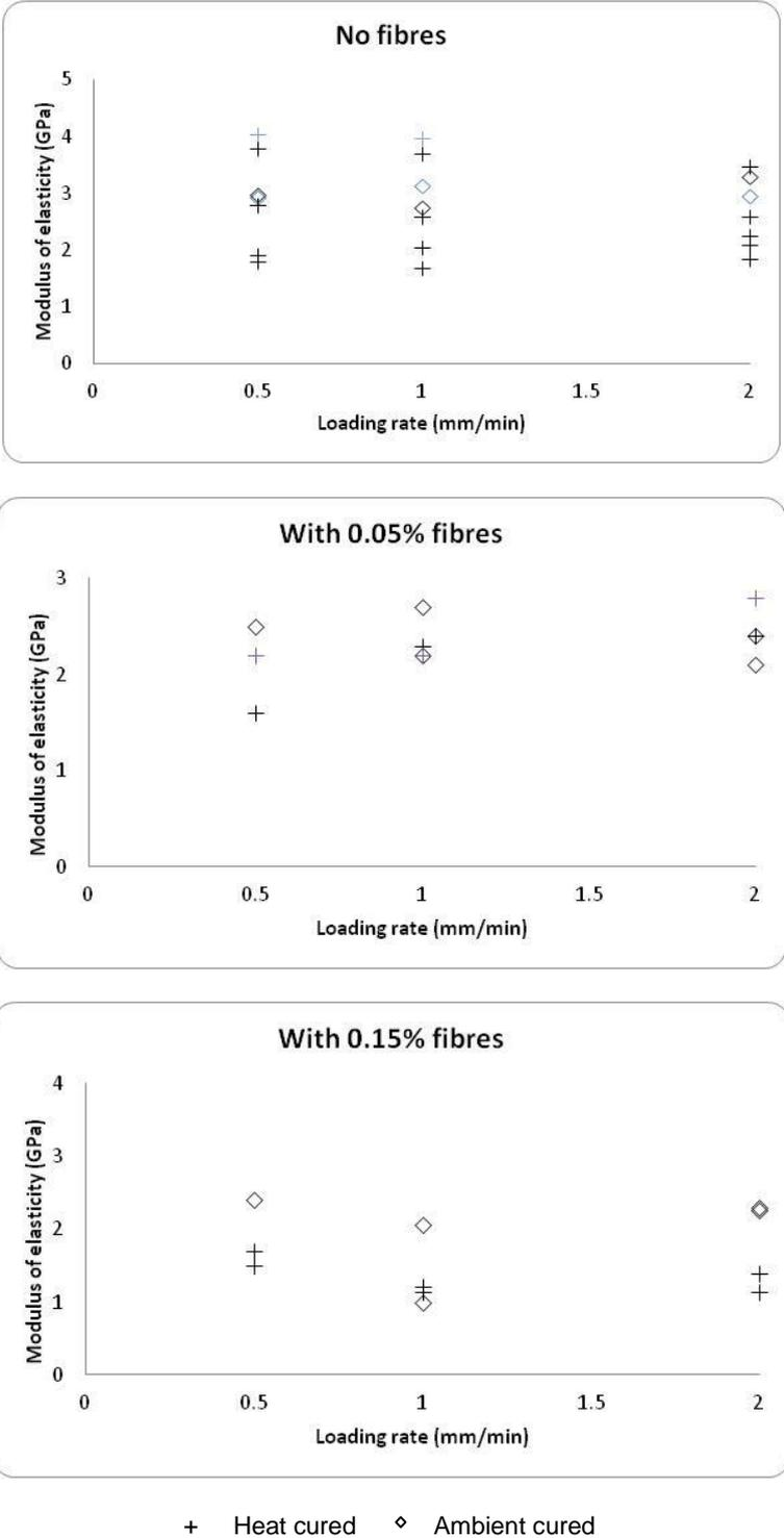
**Figure 4. Effect of fibres and strain rate on modulus of elasticity**
