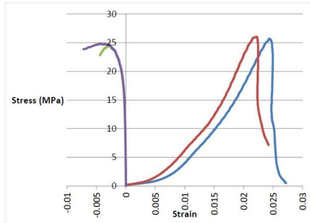
Figure 5. Typical stress-strain curve for geopolymer concrete
