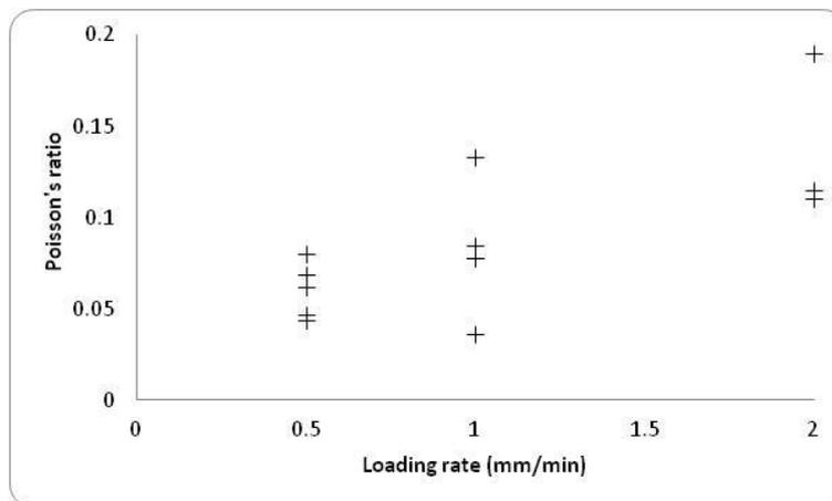
Figure 6. Effect of loading rate on poisson's ratio
