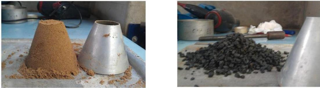
**Figure 1. SSD condition of aggregate**
