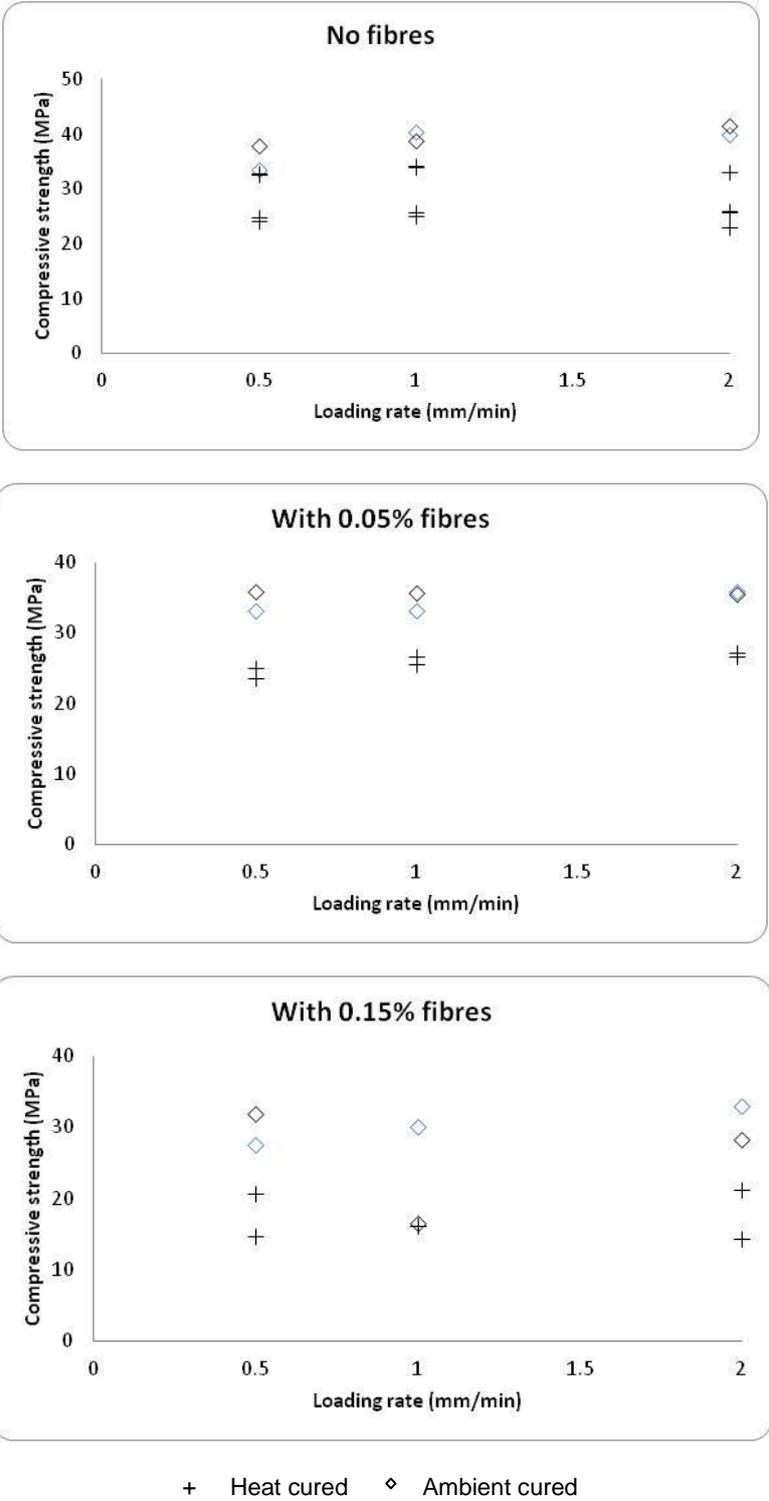
Figure 3. Effect of fibres and strain rate on compressive strength
