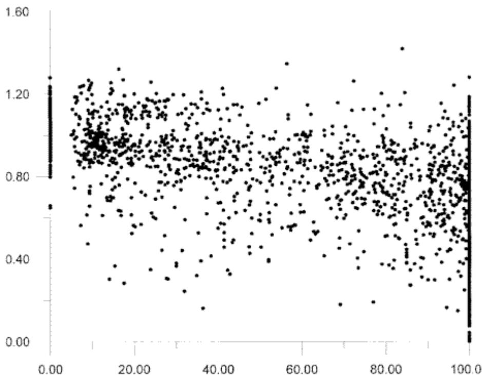
**Figure 2** UVB ratio versus cloud amount in the FOV of the camera (CAFOV), for a SZA range of 25 to 40°.
