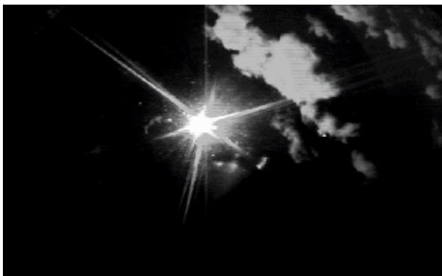
**Figure 4** CCD image taken by the SCSC on the 22<sup>nd</sup> October 1997 at 9:32 AM. This cloud configuration produced the smallest enhancement of 20 % with a SZA of 39.7 ° and a CAFOV of 39.3 %.
