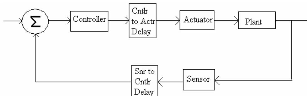
Figure 2.5 Delays in Networked Control System
