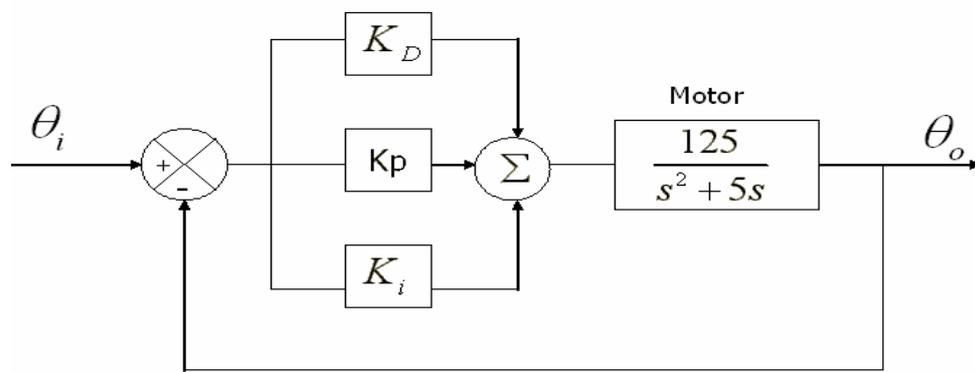
Figure 3.5 Block Diagram PID controller + Motor
