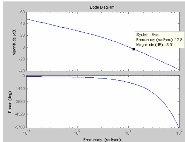
Figure 4.3 Bode Plot of the plant  $\frac{125}{s^2 + 5s}$
