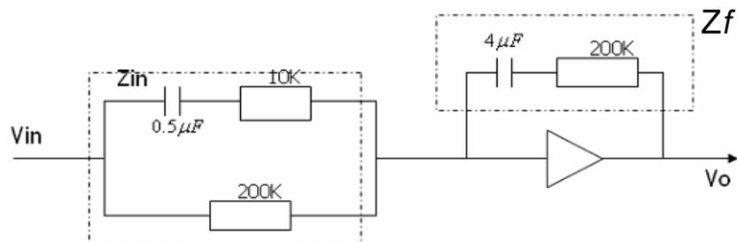
Figure 3.6 Practical PID arrangements
