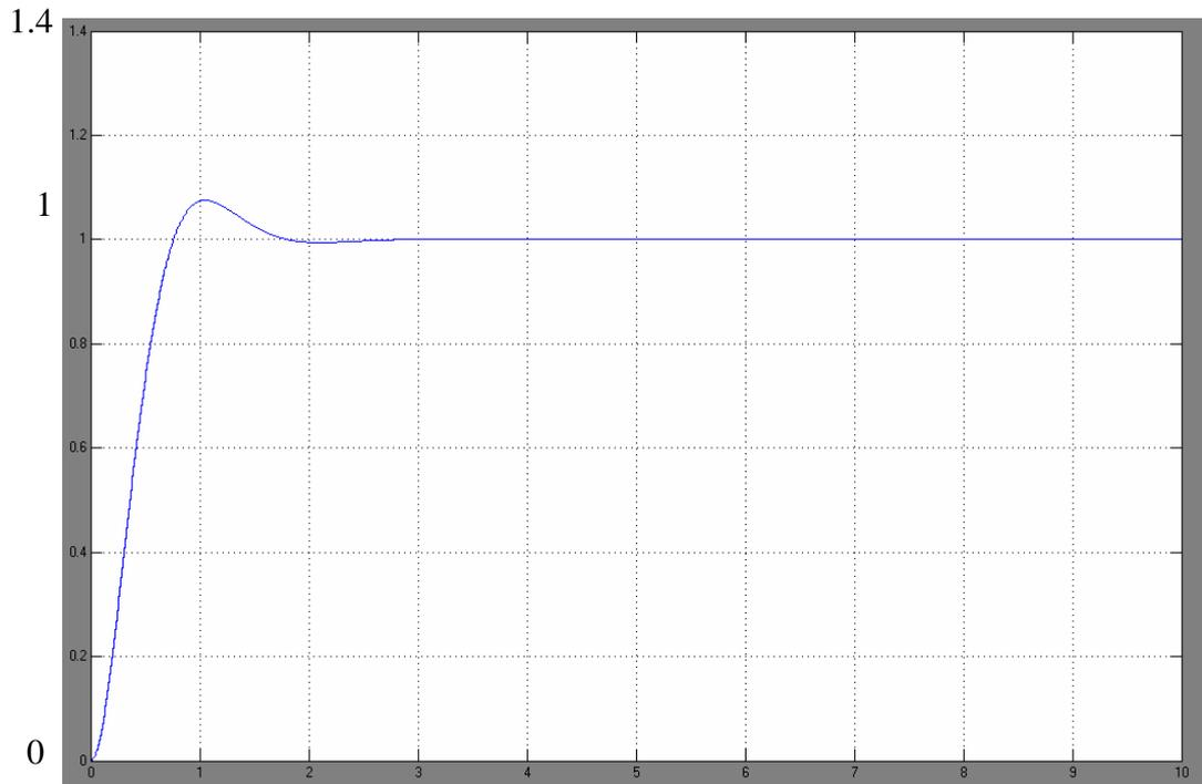
Figure 5.5 System response with  $e(k-1)$  missing and previous PID parameters values.
