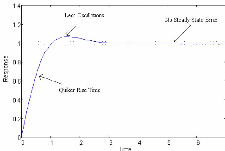
Figure 3.4 Typical PID response
