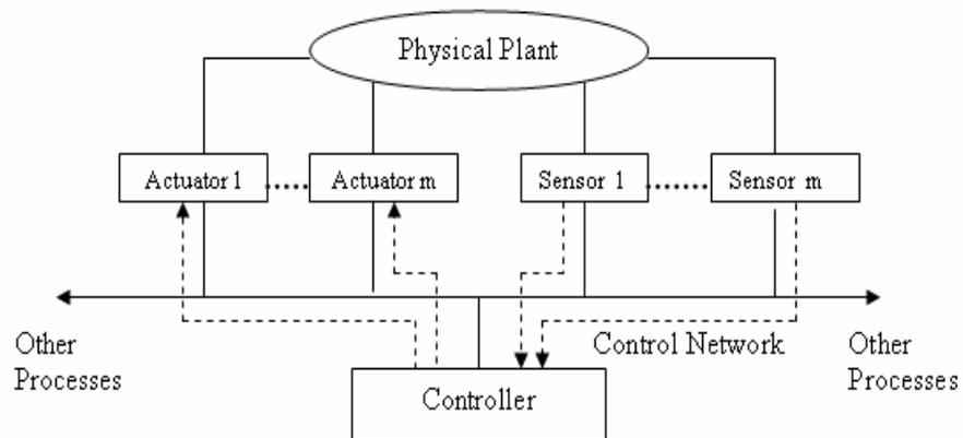
Figure 2.2 Direct Structure reproduced from (Wei Zhang 2001)
