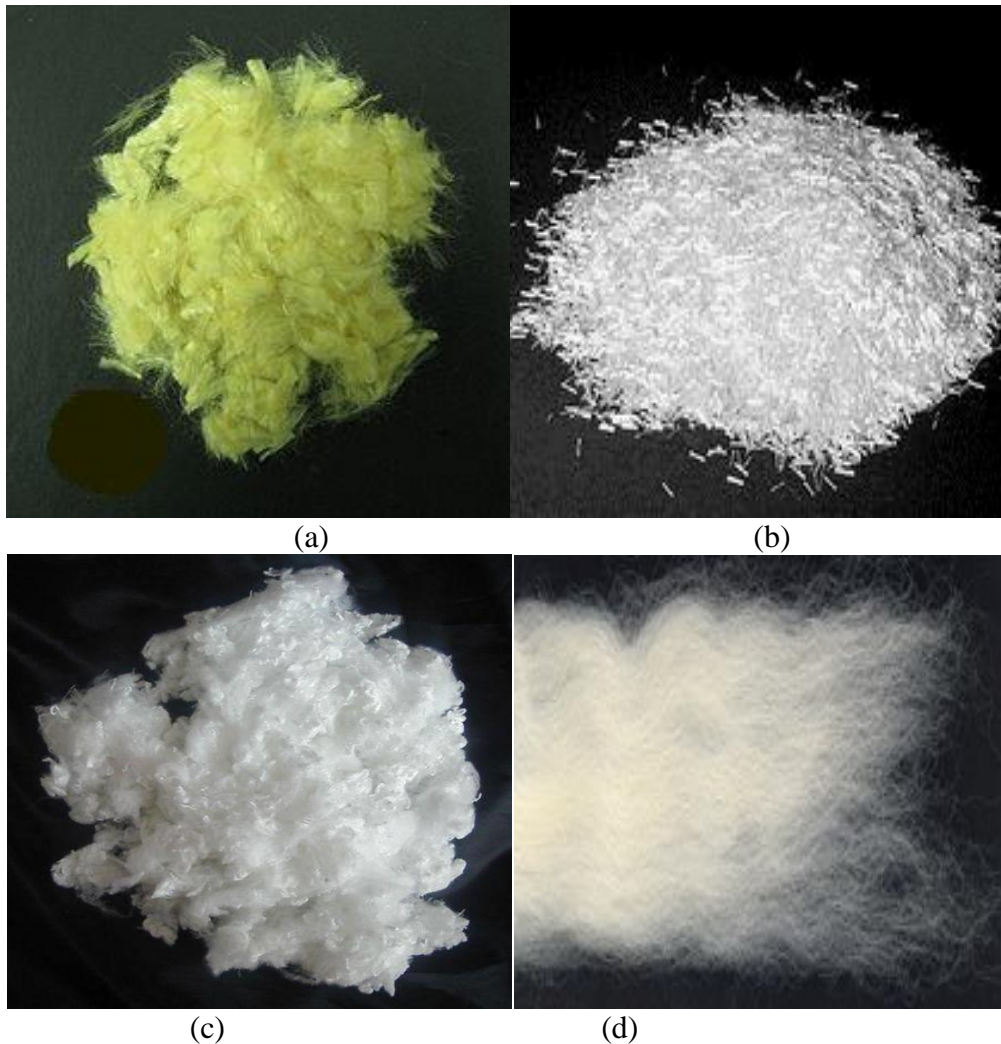
Figure 2. Examples of textile fibre; (a) Aramid, (b) Glass, (c) Cotton and (d) Wool (Kadolph & Langford, 2001).
