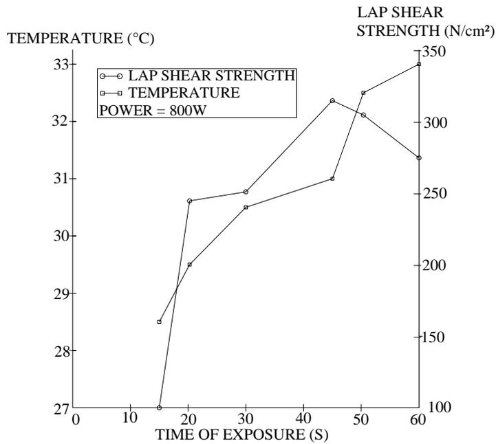
**Figure 10: Lap shear bond strength and temperature against time of exposure to microwaves of 800W in the samples of PS/GF (33%)**
