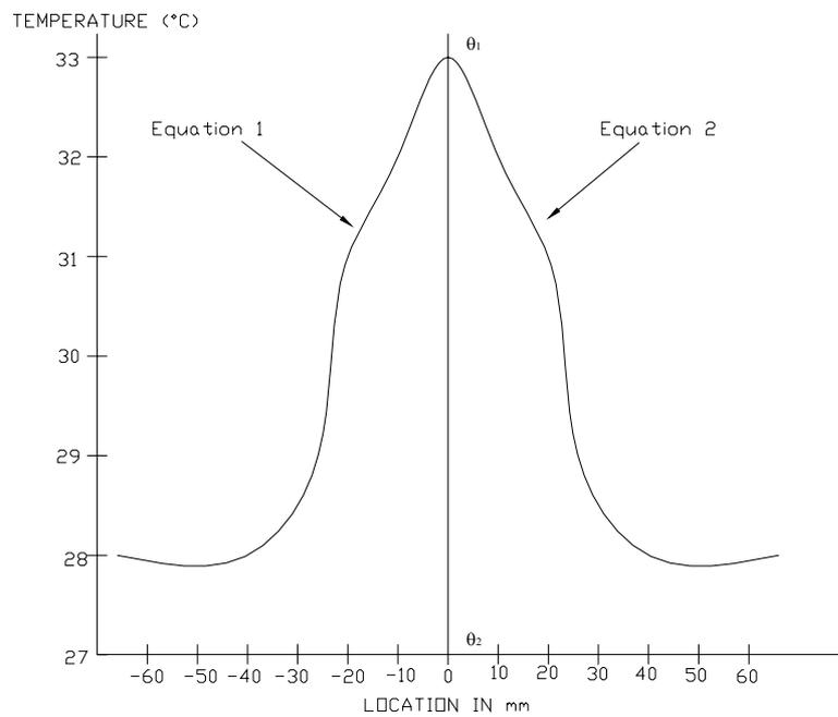
**Figure 8: Heat flow and temperature gradient of test pieces exposed to a power level of 800 W and a duration of 60 seconds.**
