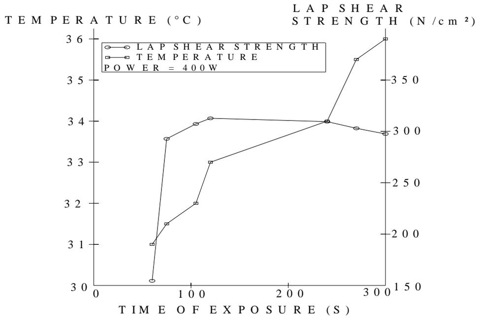
**Figure 11: Lap shear bond strength and temperature against time of Exposure to microwaves of 400W in the samples of PS/GF (33%)**
