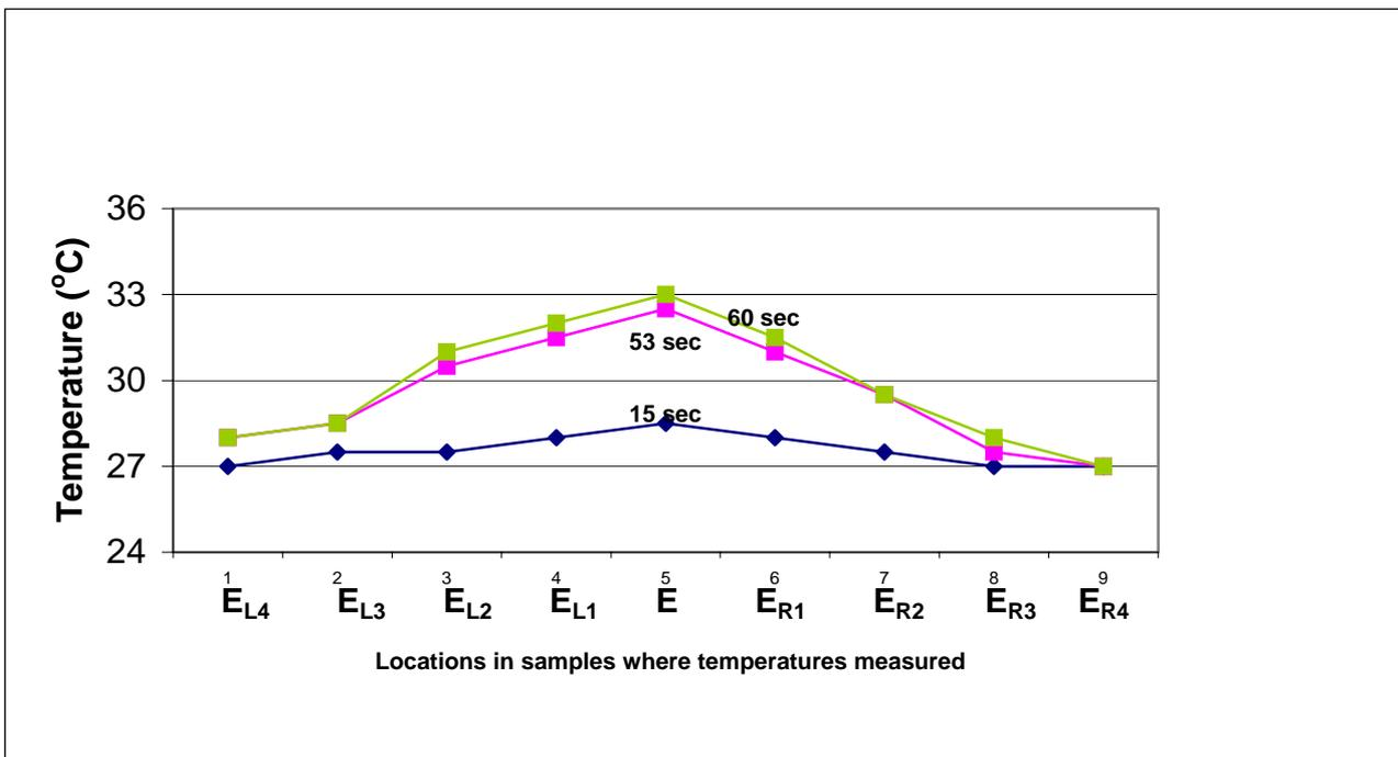
Figure 6: Temperature at different locations in samples with different exposure duration to 800 W microwave irradiation
