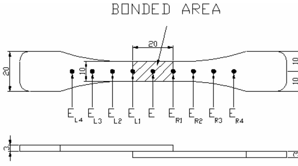
Figure 5: Locations at which temperature measurements (in the sample) are taken
