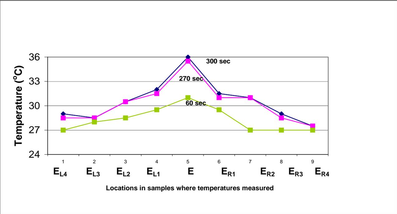
Figure 7: Temperature at different locations in samples with different exposure duration to 400 W microwave irradiation
