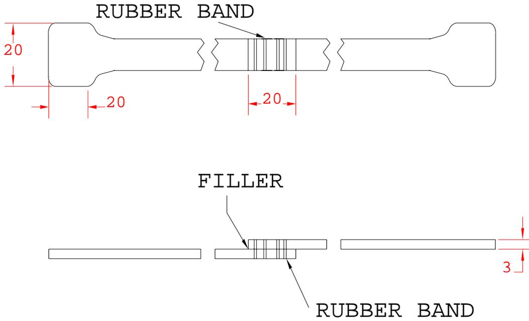
**Figure 3: Test Pieces tightened by a Dielectric Band**
