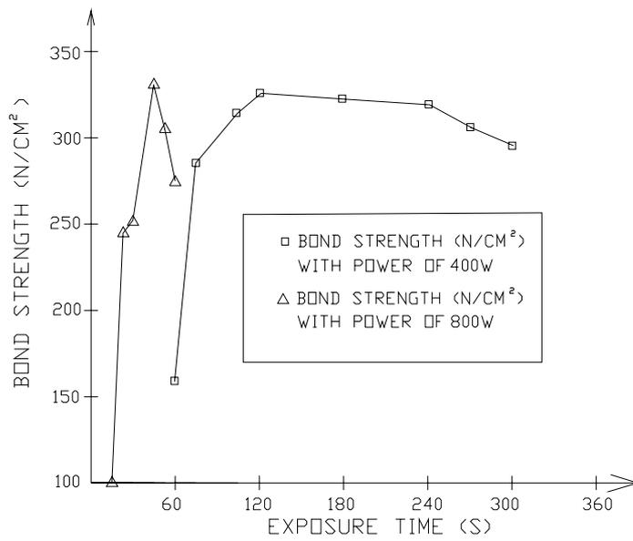
**Figure 9: Lap Shear Strength of PS/GF (33%) Joined by Fixed Frequency Microwave (2.45 GHz) in a Slotted Rectangular Waveguide using Rapid Araldite**
