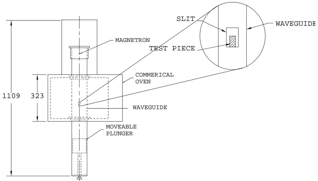
**Figure 1. Microwave Facilities Configuration**
