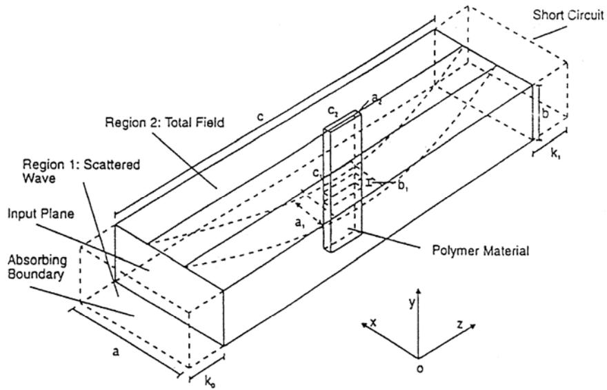
**Figure 2: A Ridge Waveguide for Microwave Heating of Polymer Materials**
