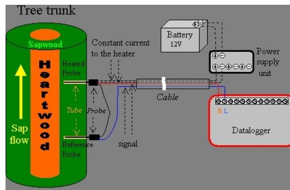
Figure 2.11: Schematic of Granier's thermal dissipation sap flow sensors
