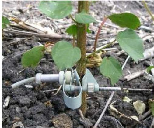
Figure 2.7: Dendrometer measuring stem diameter fluctuations
