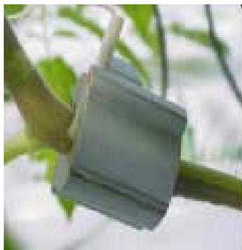
Figure 2.8: SF-4 - Stem flux relative rate sensor
