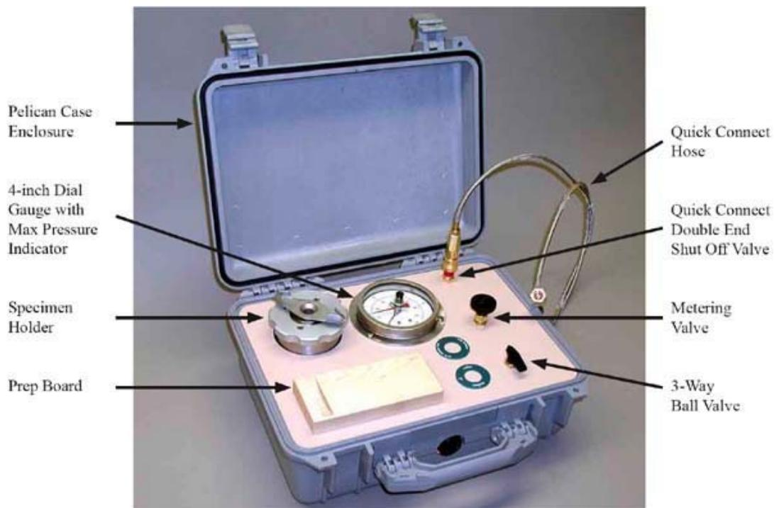
Figure 2.1: Portable pressure chamber and console
