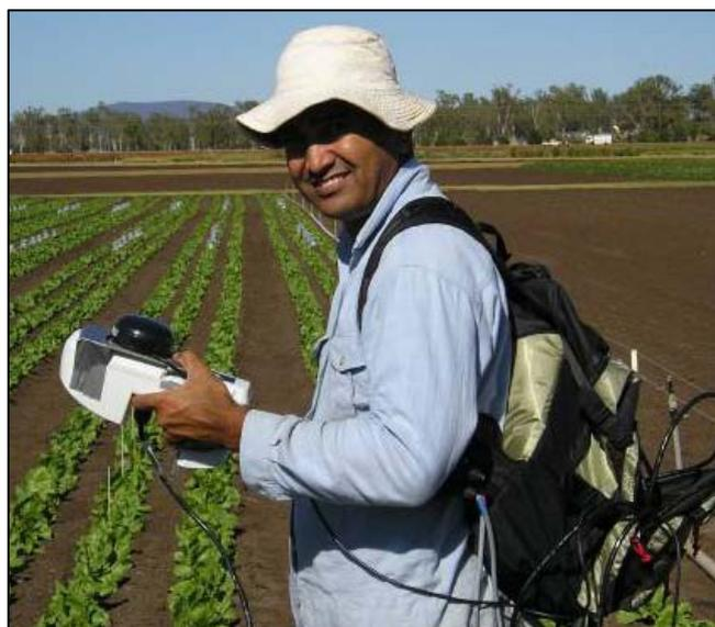
Figure 3.2: NDVI Greenseeker sensor with logger in backpack.
