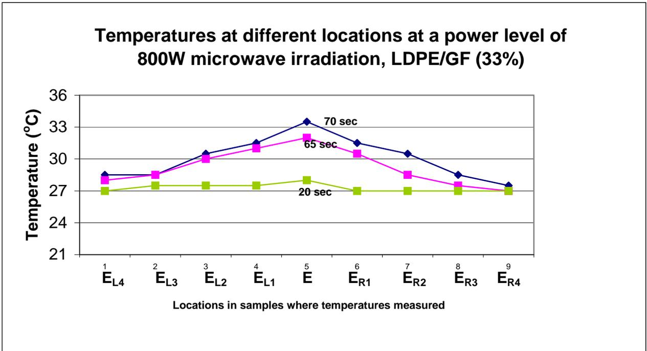
Figure 5: Temperature at different locations in samples with different exposure duration to 800 W microwave irradiation
