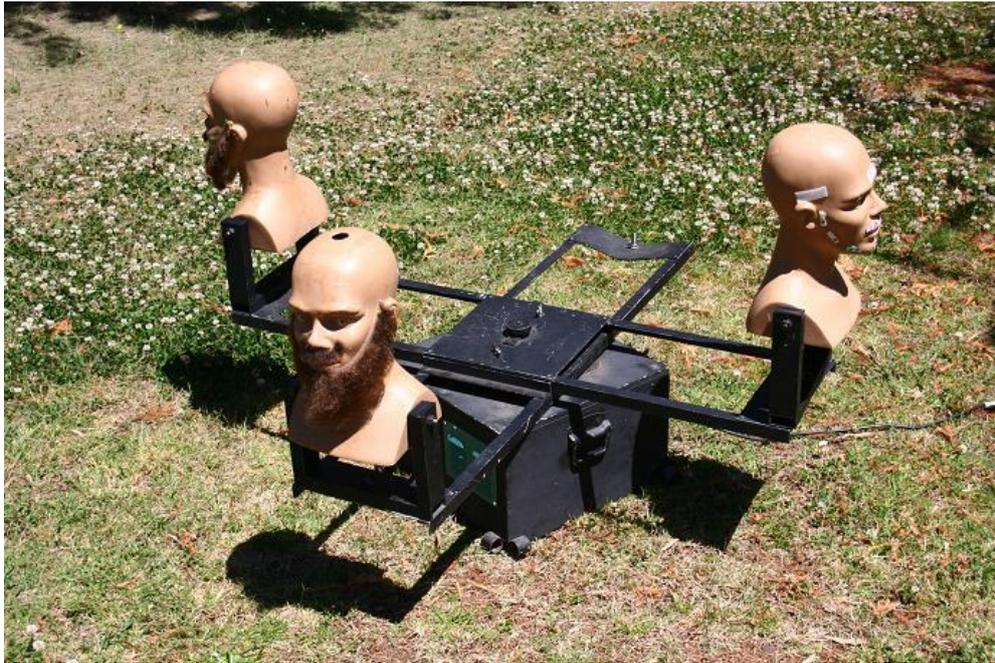
Figure 1 – The experimental set up for the dosimetric measurement of the UV protection provided by facial hair showing the rotating platform, the manikin head with the long beard, the short beard and with no beard.
