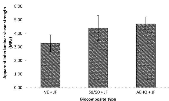
Fig. 7 Interlaminar shear strength of biocomposite samples
