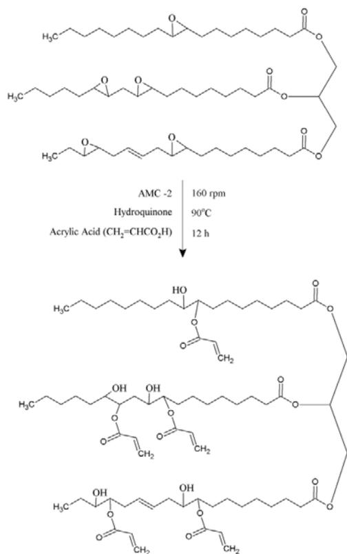
Fig. 2 *In situ* acrylation of epoxidized hemp oil
