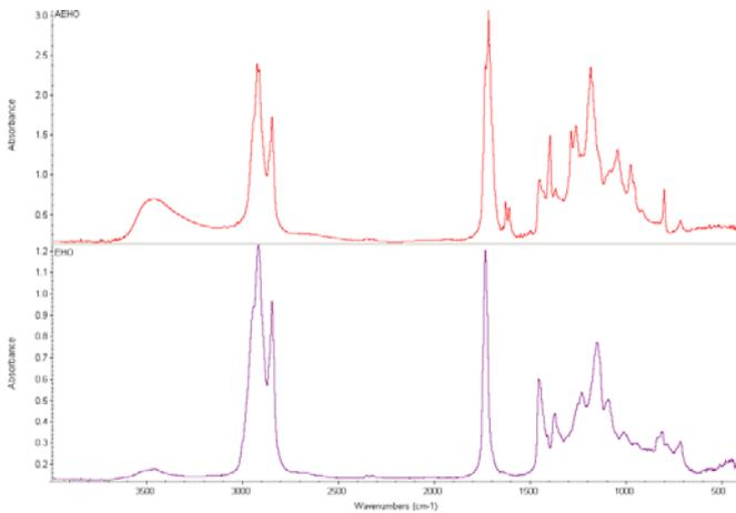
Fig. 4 FTIR spectra obtained from EHO and AEHO
