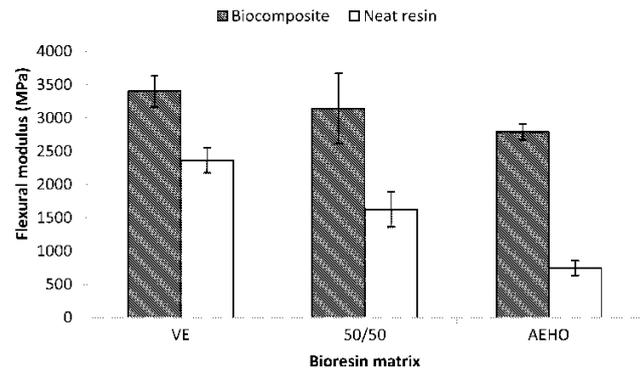
Fig. 5 Flexural modulus of bioresin and biocomposite samples
