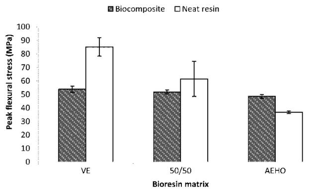
Fig. 6 Flexural strength of bioresin and biocomposite samples
