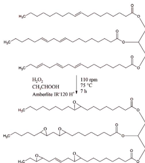
Fig. 1 *In situ* epoxidation of hemp oil
