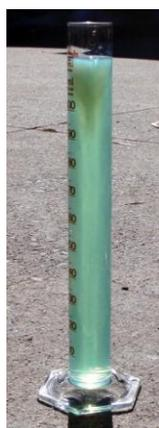
***Figure 2: The cyanotype aqueous solution exposed to sunlight in a large measuring cylinder shows the beginnings of the blueprint reaction near the top of the cylinder. Mixing processes caused by variations in compound densities take place during an exposure event, eventually influencing the colour of the entire tube.***
