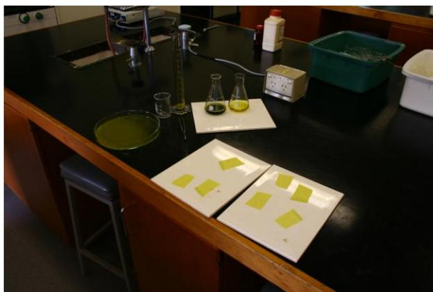
***Figure 1: Cyanotype cloth dosimeters placed on a ceramic tile for drying prior to an exposure experiment. A large Petri dish was used for soaking the dosimeters and can be seen in the left of the image.***
