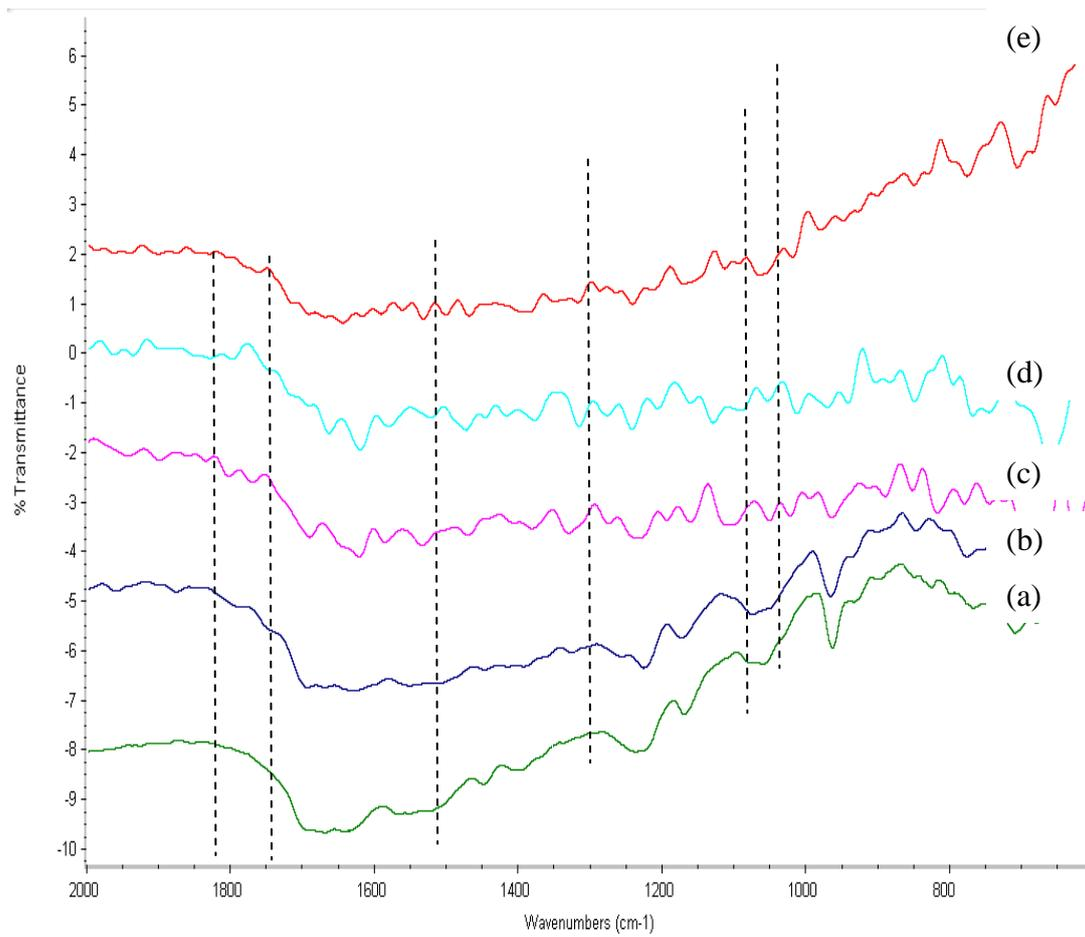
Figures 5. FTIR spectra of tussah silk fibre degummed for (a) 0 minute (control sample), (b) 15 minutes, (c) 30 minutes, (d) 45 minutes and (e) 60 minutes.
