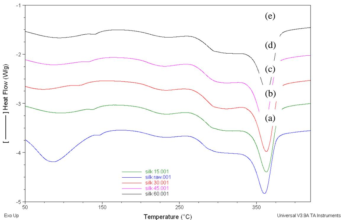
Figure 2. DSC curves of tussah silk fibres degummed for (a) 0 minute (control sample), (b) 15 minutes, (c) 30 minutes, (d) 45 minutes and (e) 60 minutes.
