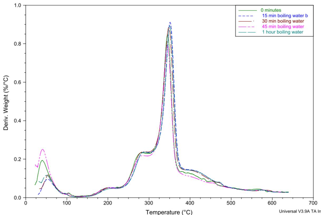
Figure 4. DTG curves of the tussah silk fibres degummed for (a) 0 minute (control sample), (b) 15 minutes, (c) 30 minutes, (d) 45 minutes and (e) 60 minutes.
