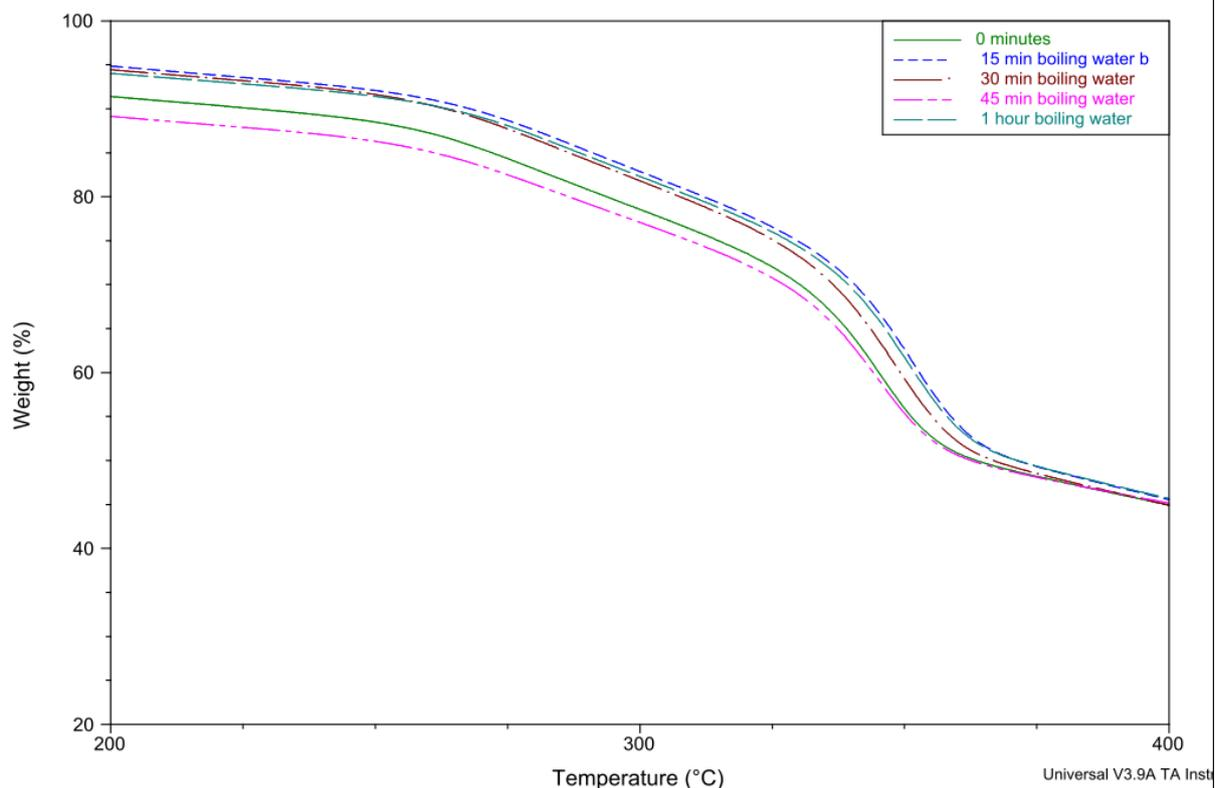
Figure 3. Thermogravimetric curves of the silk fibres degummed for (a) 0 minute (control sample), (b) 15 minutes, (c) 30 minutes, (d) 45 minutes and (e) 60 minutes.
