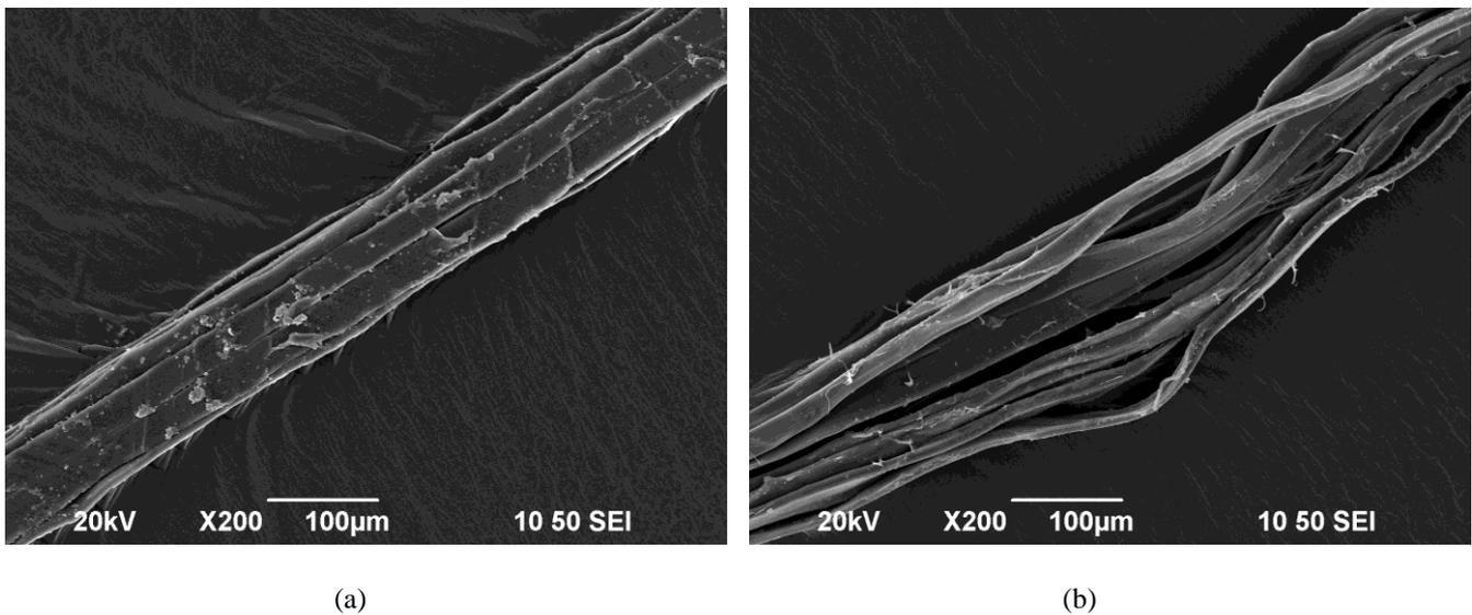
Figure 1. Surface of (a) raw silk fibres and (b) degummed silk fibre.
