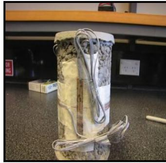
Figure 1. Permeable concrete sample with strain gauges.
