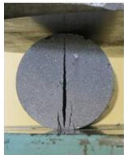
Figure 3. Split tensile testing.
