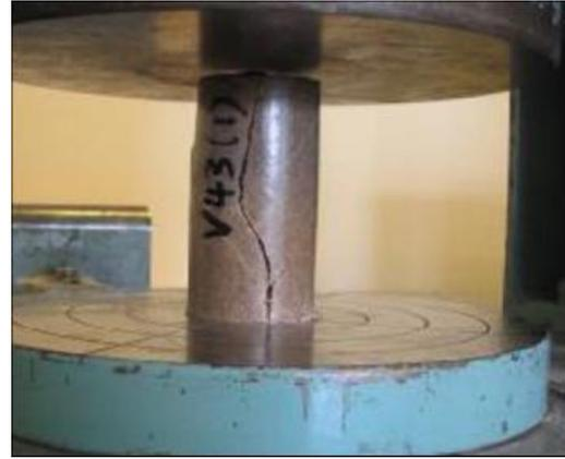
Figure 1. Compressive strength testing.
