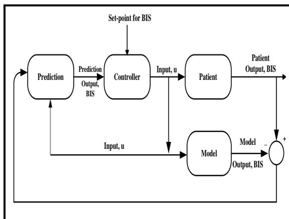
Figure 4 – The model predictive control simulation design
