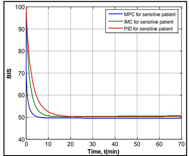
**Figure 7** – The performance of MPC, IMC and PID controllers for sensitive patient
