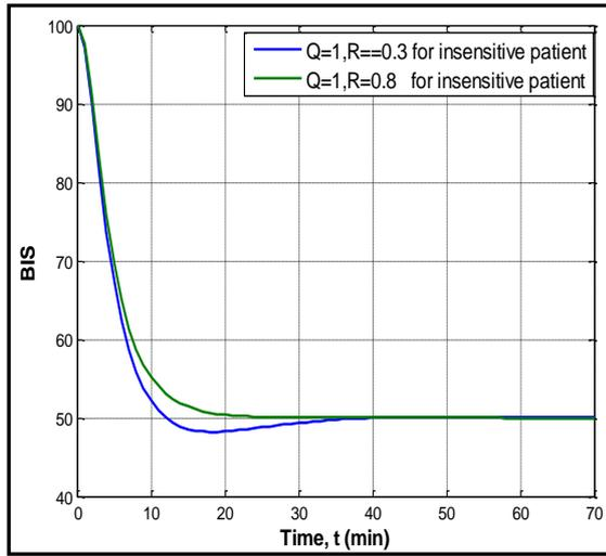
**Figure 6** – MPC controller performance for different R and Q weights
