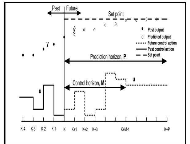
Figure 3 – The basic concept of model predictive control
