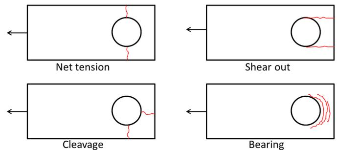
Figure 5. Failures mechanism of FRP mechanical connector
