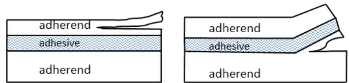
Figure 7. Typical FRP bonded joints failure
