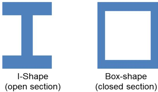
Figure 6. Example of open and closed section
