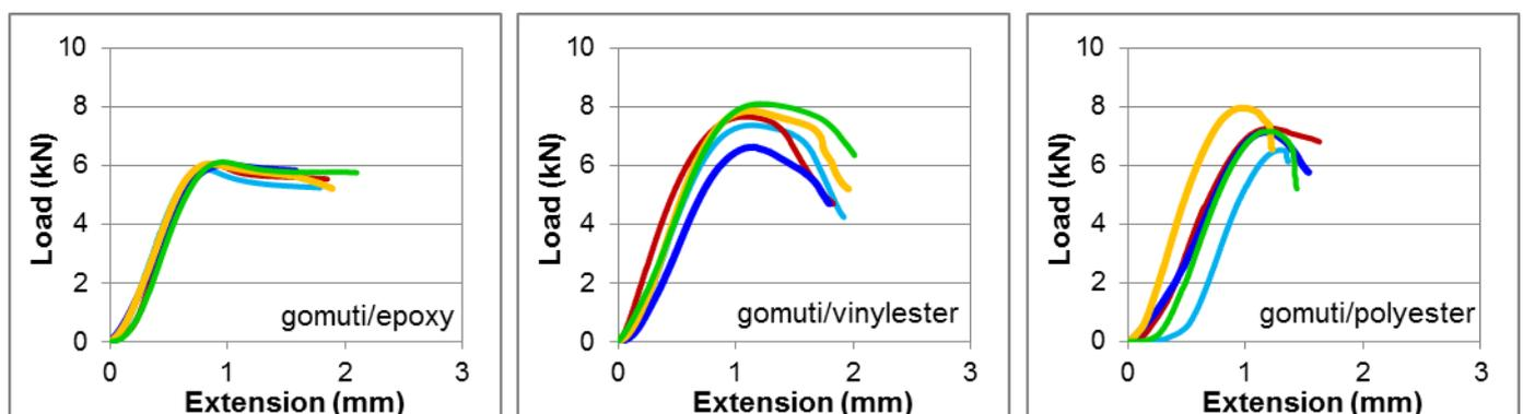
Figure 5. Load vs extension plots of compressive specimens
