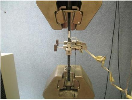
Figure 2. Tensile test set-up
