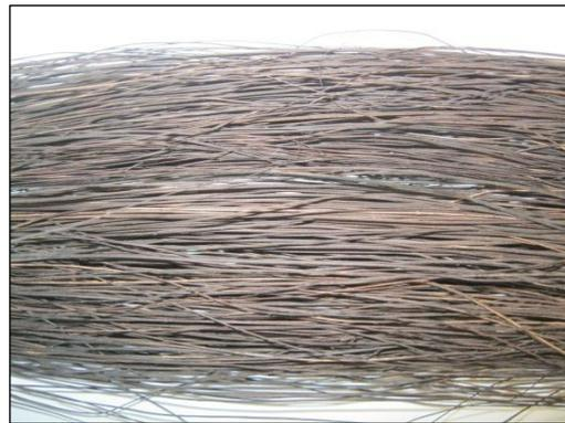
Figure 1. Unidirectional aligned gomuti fibre
