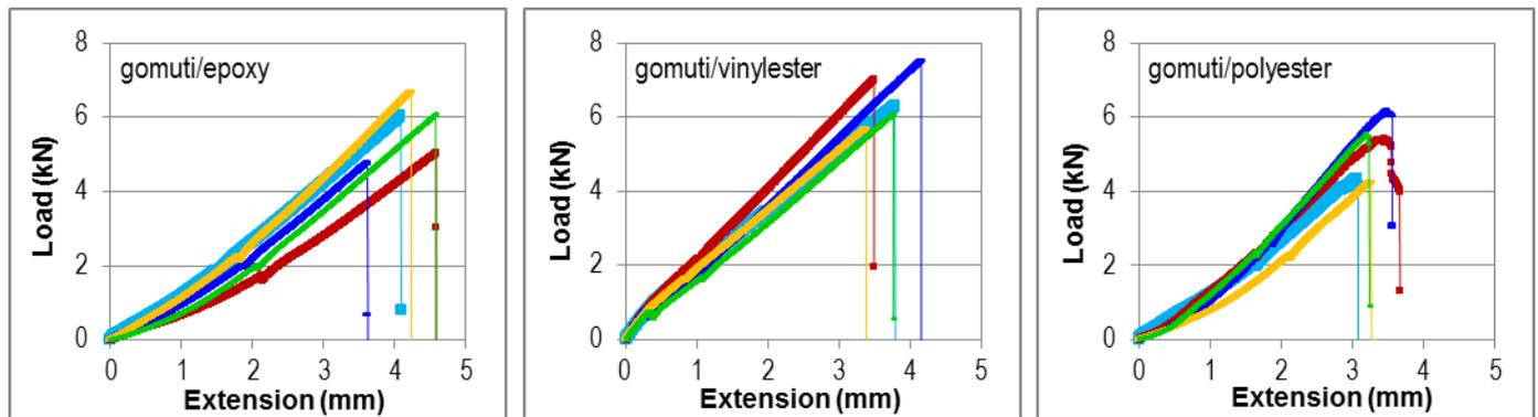
Figure 4. Load vs extension plots of tensile specimens
