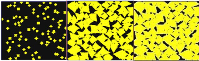
Figure.3. Microstructure formation and evolution in Al-6%Si alloy at a pouring temperature of 620°C.  $t=100, 150$  and  $300s$ , calculation domain:  $1mm \times 1mm$
