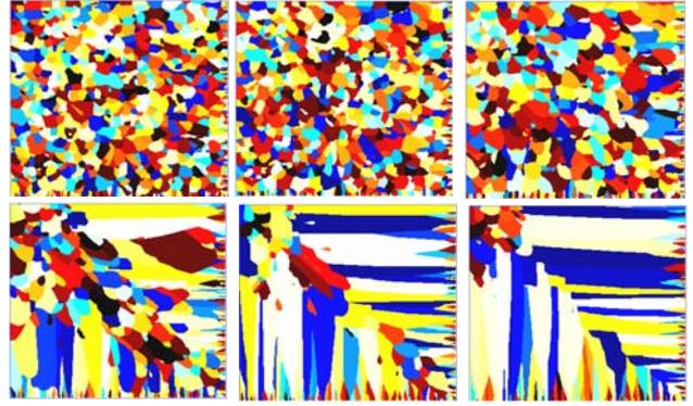
Figure 1. Effect of mould preheat temperature on microstructure formation in Al-1%Si alloy, T=25, 100, 300, 350, 400, 500 °C
