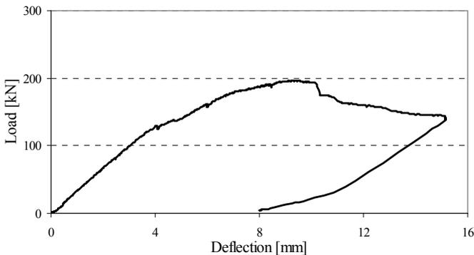
Figure 4. Load – Deflection curve of the control beam, RCB1
