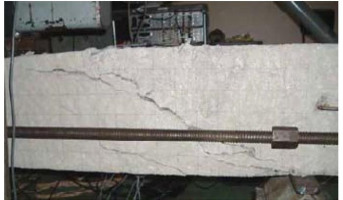
Figure 6. Failure of the control beam, RCB2
