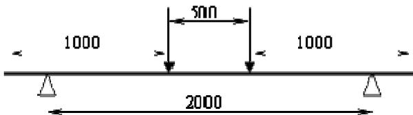
Figure 1b. Typical loading arrangement for the beam
