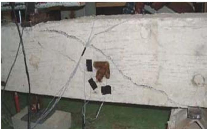
Figure 5. Failure of the control beam, RCB1
