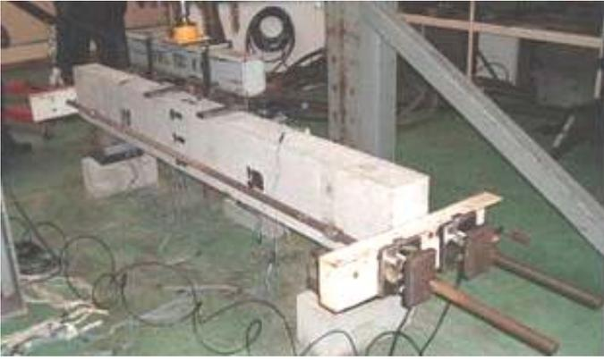
Figure 3b. Experimental setup for the post-tensioned beam
