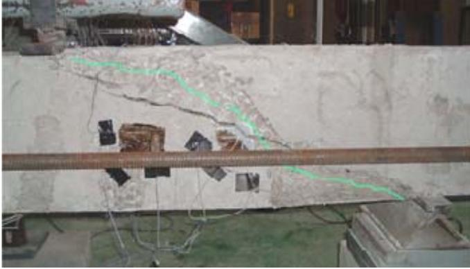
Figure 8. Failure of the control beam, RCB3 (initial crack is highlighted)
