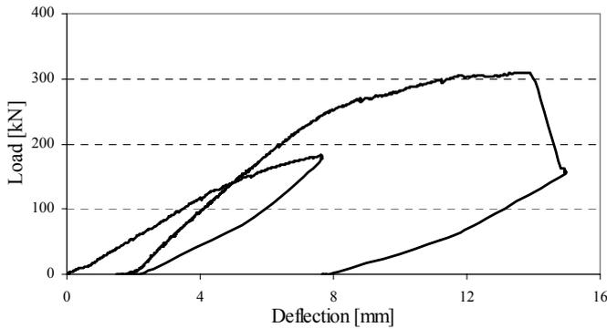
Figure 9. Load – Deflection curve of the control beam, RCB3
