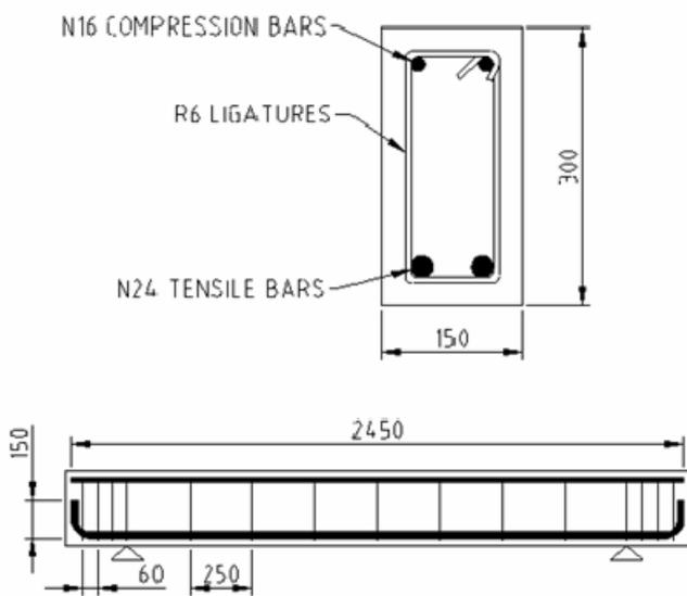
Figure 1a. Typical reinforcement layout of the beam
