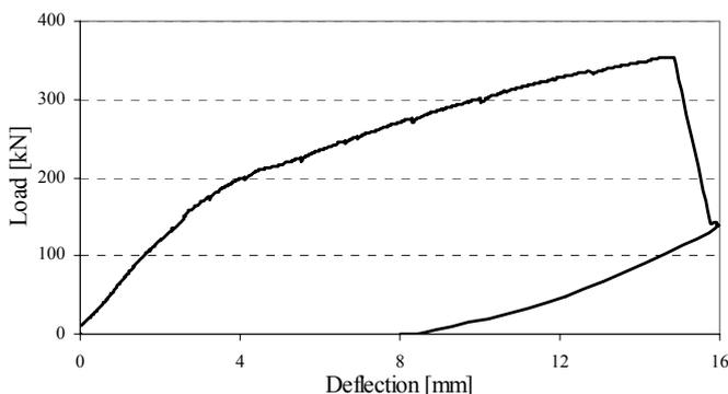
Figure 10. Load – Deflection curve of the control beam, RCB4
