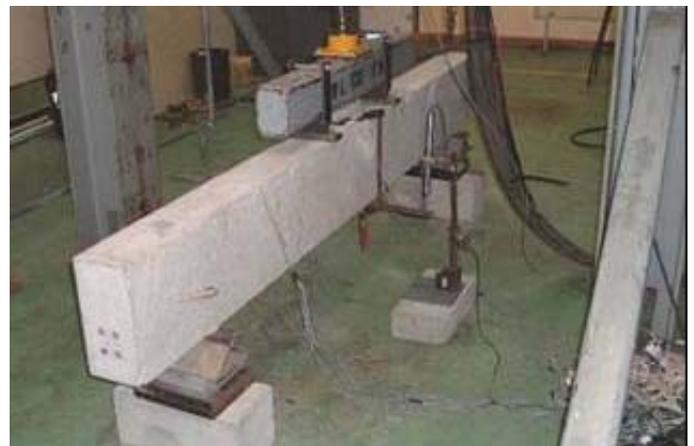
Figure 3a. Experimental setup for the control beam
