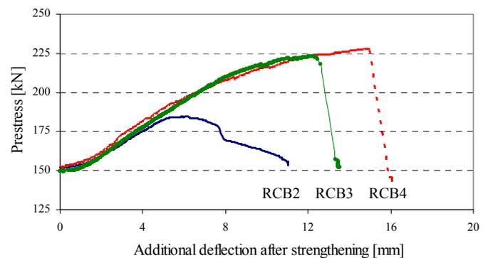
Figure 11. Increase in external prestressing force with deflection of the beams
