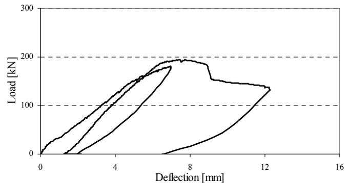
Figure 7. Load – Deflection curve of the control beam, RCB2
