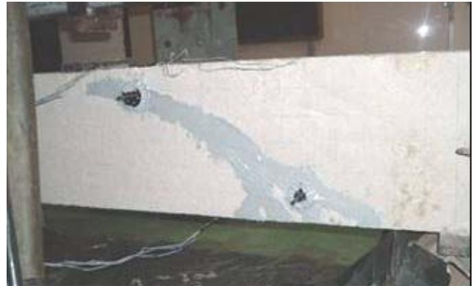
Figure 2. Repaired shear crack using epoxy injection
