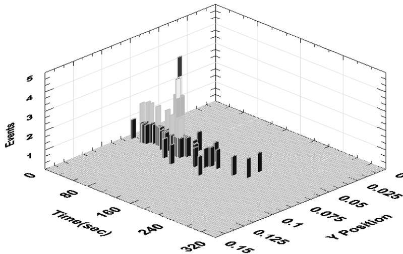
Figure 3: AE events at crack location; near notch.
