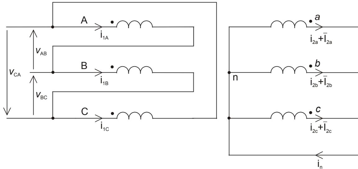
Figure 11: 3-phase transformer with DC injection.
