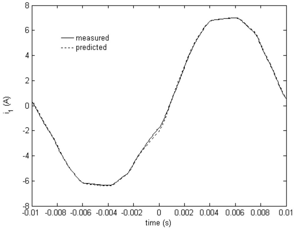
Figure 5. Primary current waveforms with unity power factor load.
