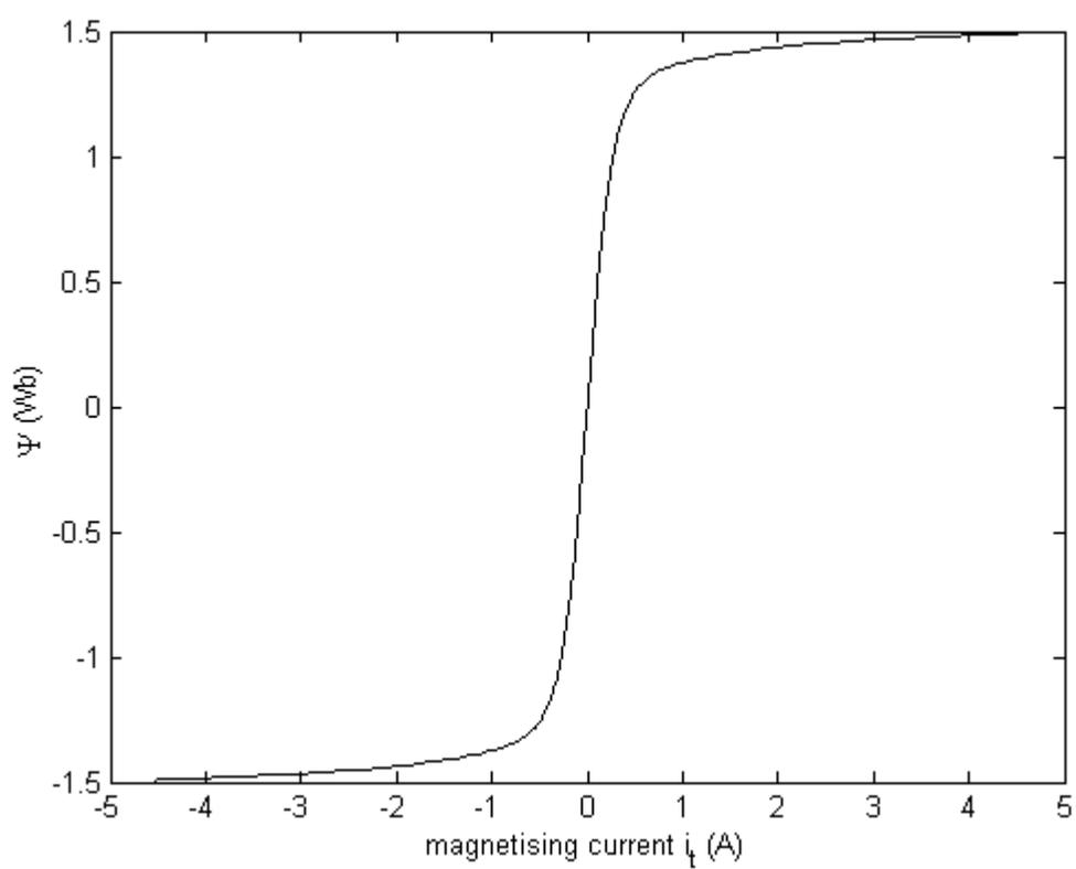
Figure 3: Magnetising curve deduced from Figure 2 and equation (6).
