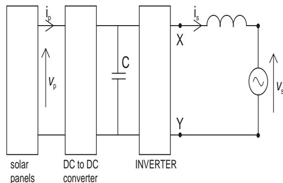
Figure 1: Grid-Connected PV System
