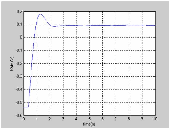
Figure 9: Measured Compensating Current Signal (one inductor directly across AC supply)
