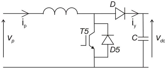
Figure 2: DC to DC Converter
