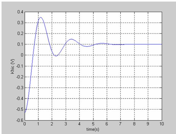
Figure 8: Predicted Compensating Current Signal
