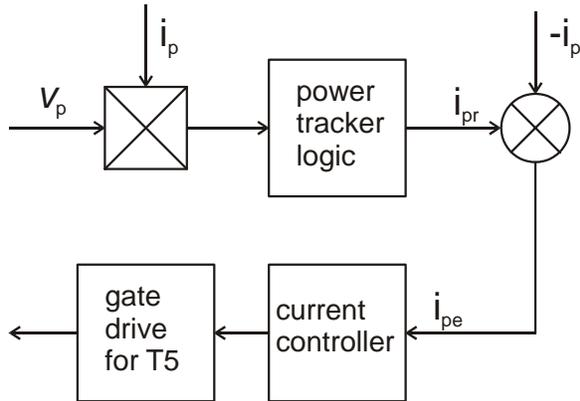
Figure 3: Block Diagram of Maximum Power Tracker
