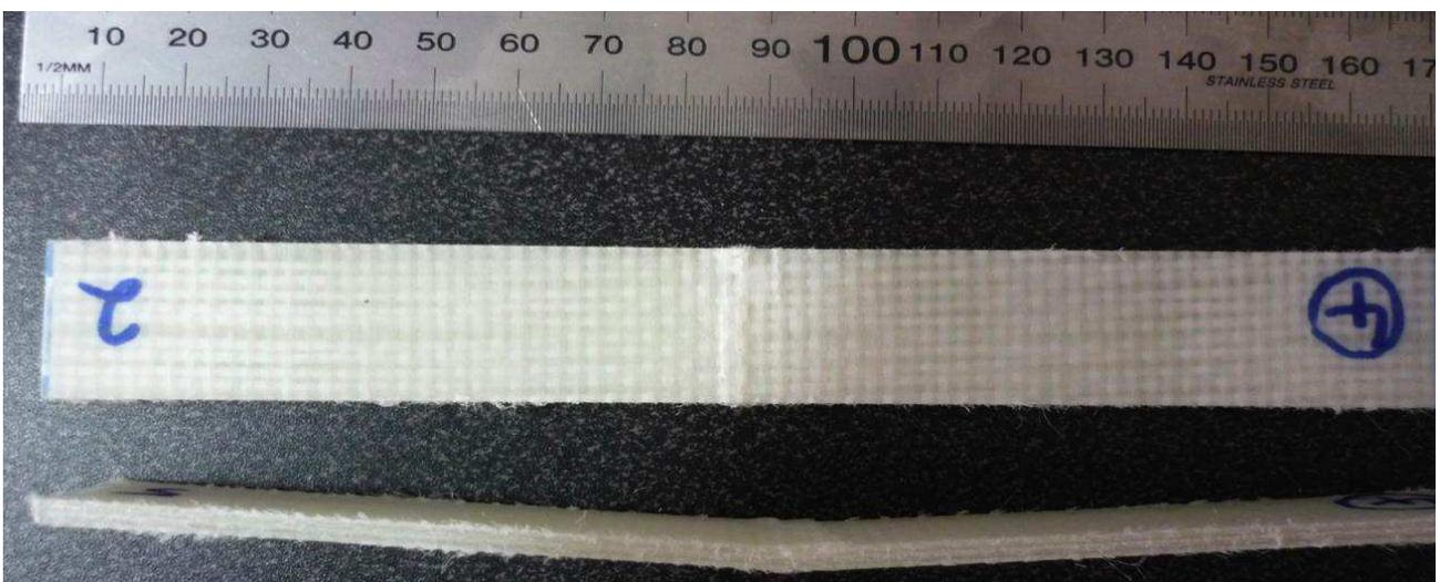
**Figure 9. Impact damage of a GI/HMPP 410-2 specimen.**
