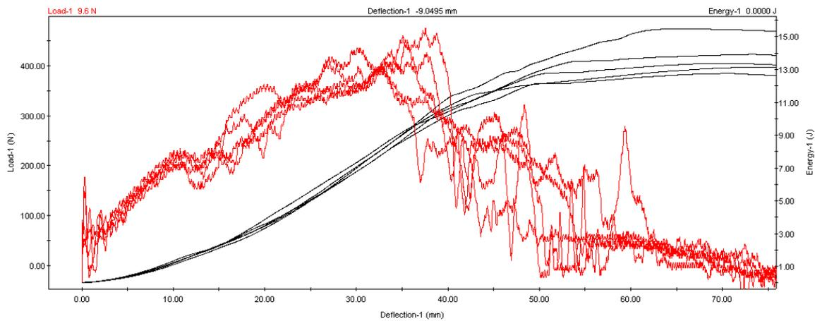
Figure 2. The contact force and the energy absorption of HMPP410 specimens with deflection.
