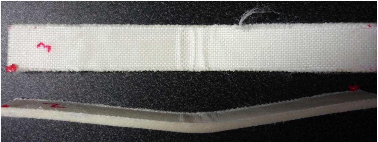
**Figure 7. Impact damage of a HMPP 150 specimen.**
