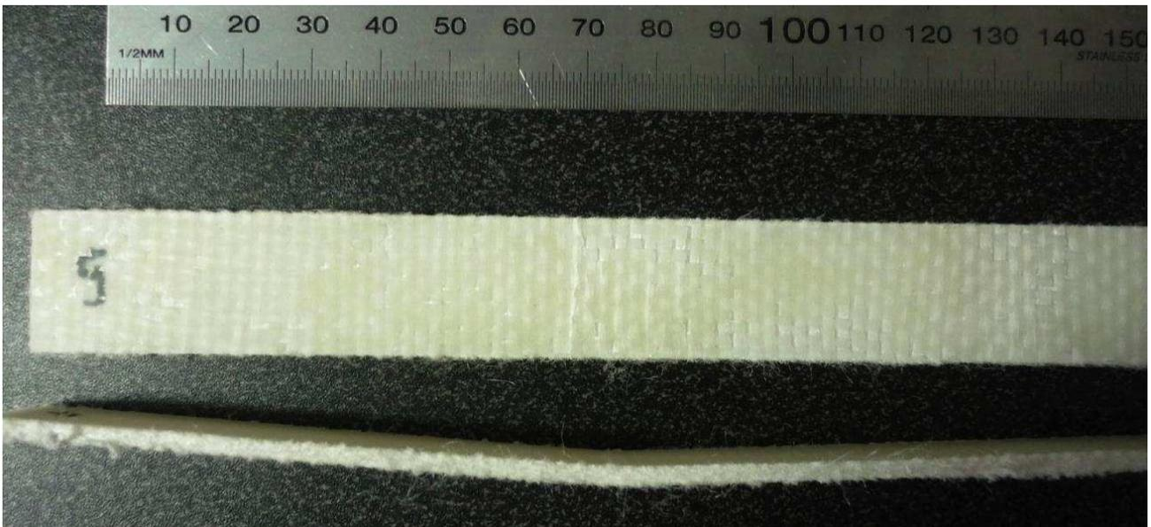
**Figure 8. Impact damage of a HMPP 410 specimen.**
