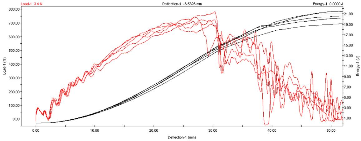
Figure 4. The contact force and the energy absorption of GI/HMPP410-2 specimens with deflection.
