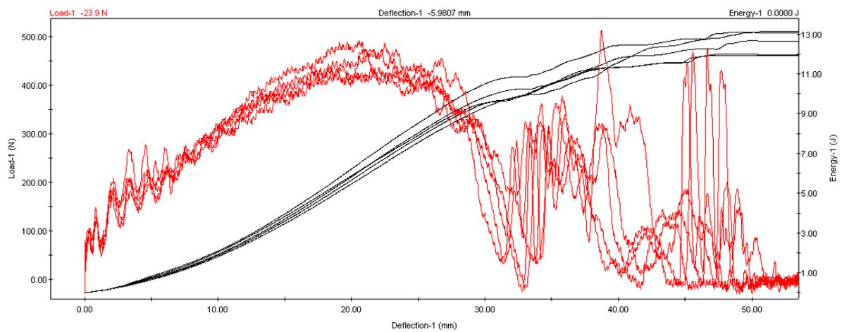
Figure 6. The contact force and the energy absorption of GI/HMPP\_GO specimens with deflection.
