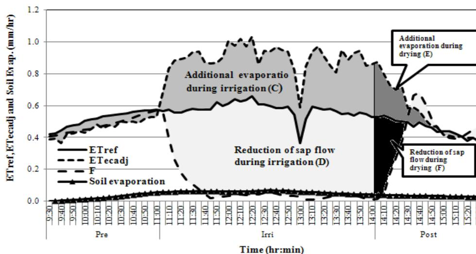
Figure 1: Components of total ET measured by ECV-sap flow method during sprinkler irrigation
