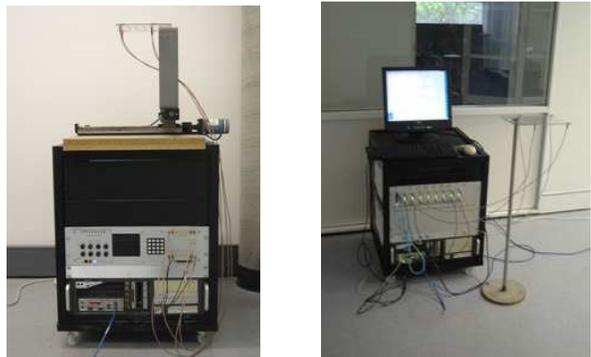
Figure 1: CSIRO ICT center MIMO-OFDM channel sounder (Left: Tx, Right Rx)
