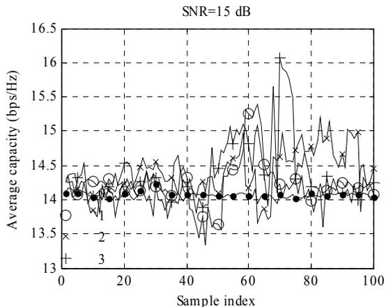
Figure 5. MIMO channel capacity for LoS measurements.
