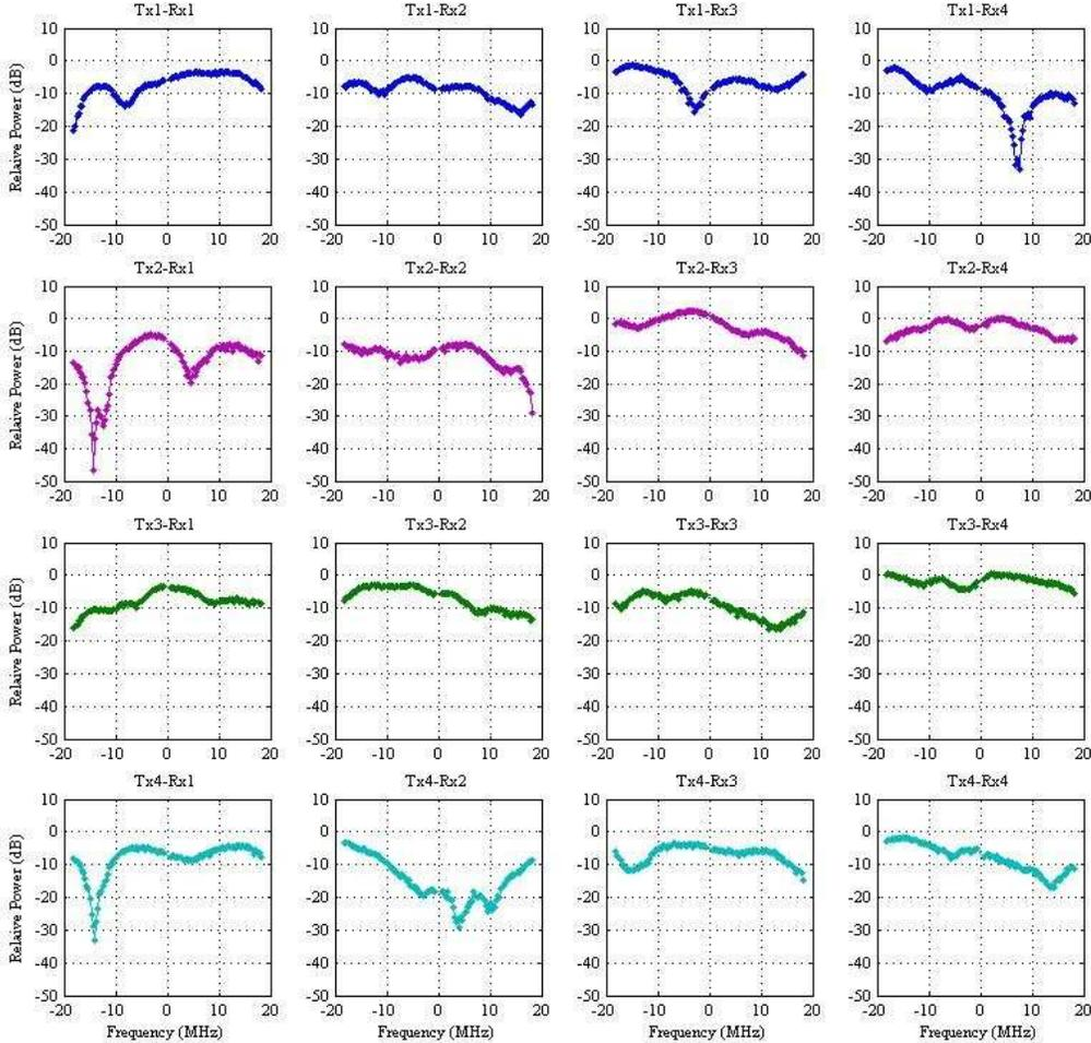
Figure 3. A sample of the 4X4 MIMO-OFDM sub-channels
