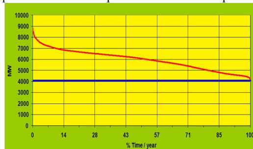
Fig.3. Occurrence of electrical energy demand in Queensland during 2010. peak demand 8890.66 MW, base-load 4055 MW and total supplied electrical energy 52.324 TWh. Data extracted from the Australian Energy Market Operator.
