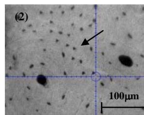
Fig.2 A total of 600 indentations were produced within 15 specimens in 5 randomly chosen interstitial lamellae along longitudinal direction of the bovine cortical bone.
