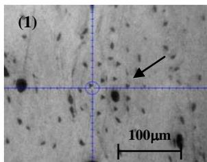
Fig.1 A total of 600 indentations were produced within 15 specimens in 5 randomly chosen osteons lamellae along longitudinal direction of the bovine cortical bone.
