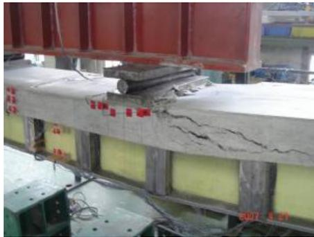
(a) Compression failure of NSC slab
