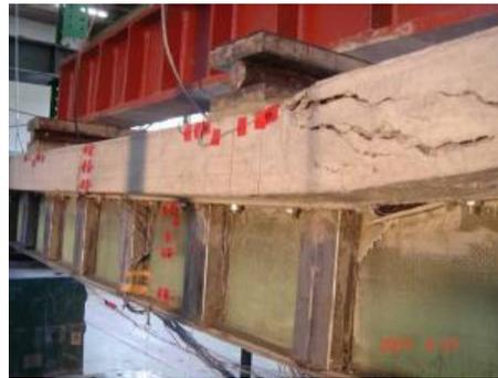
(b) Shear failure of HFRP beam
