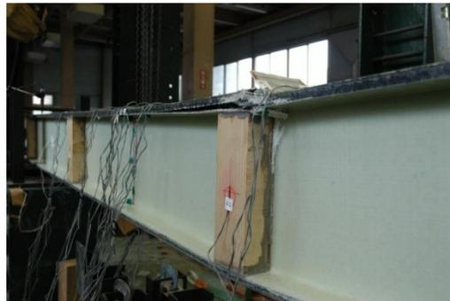
**Figure 4**—Crushing of fibers and delamination
