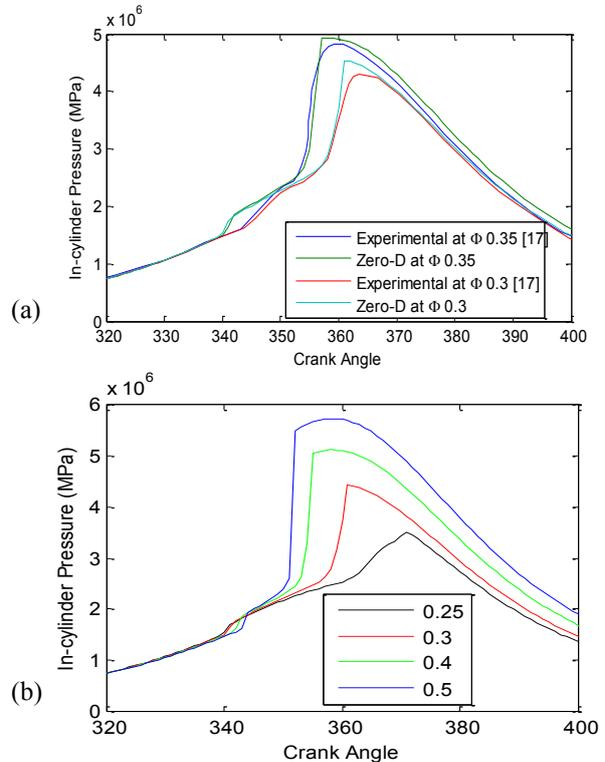
**Figure 3** Effect of equivalence ratio on the in-cylinder pressure: CR=10.0, N=900 rpm,  $T_{in}=40^{\circ}\text{C}$ ,  $P_{in}=95\text{ kPa}$  (a) Validated varying equivalence ratio; (b) Predicted in-cylinder pressure trend.
