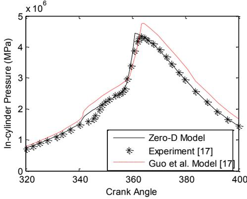
**Figure 1** Comparison between single-zone zero-dimensional model with experiment and another single-zone model using modified Woschni heat transfer model [17]. CR=10.0, N=900 rpm,  $T_{in}=40^{\circ}\text{C}$ ,  $P_{in}=95\text{ kPa}$ , AFR=50.
