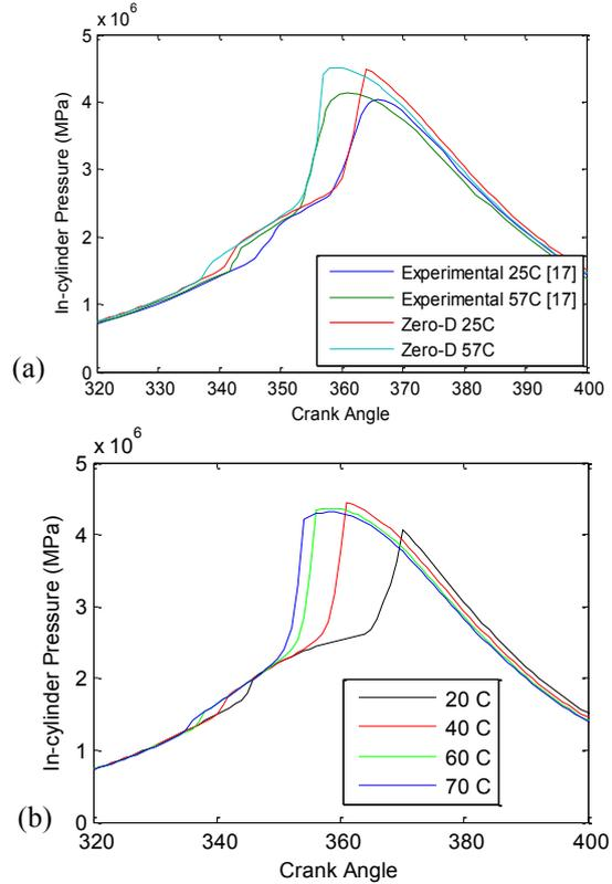
**Figure 2** Effect of intake temperature on the in-cylinder pressure: CR=10.0, N=900 rpm,  $P_{in}=95\text{ kPa}$ , AFR=50 (a) Validated varying intake temperature; (b) Predicted in-cylinder pressure trend.
