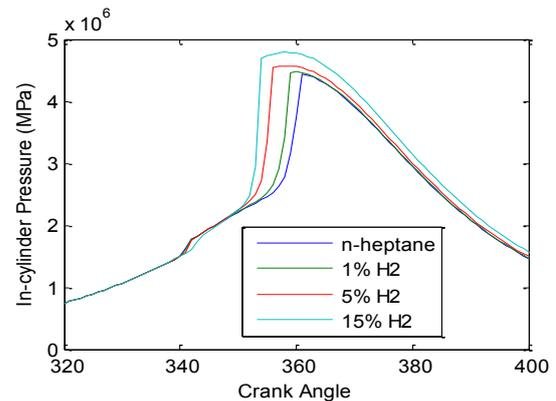
Figure 4 Predicted effect of hydrogen addition on the in-cylinder pressure for fixed n-heptane injection: CR=10.0, N=900 rpm,  $T_{in}=40^{\circ}\text{C}$ ,  $P_{in}=95\text{ kPa}$
