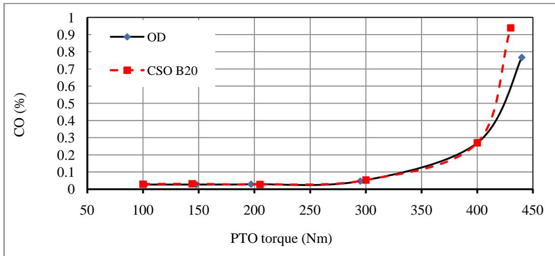
**Figure 7.** The relationship between PTO torques (Nm) and CO (%) for CD and CSO-B20
