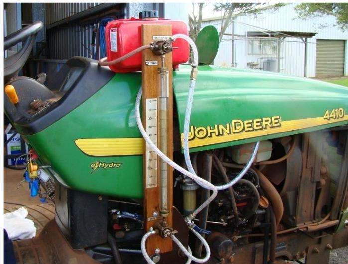
**Figure 2.** The fuel measurement system
