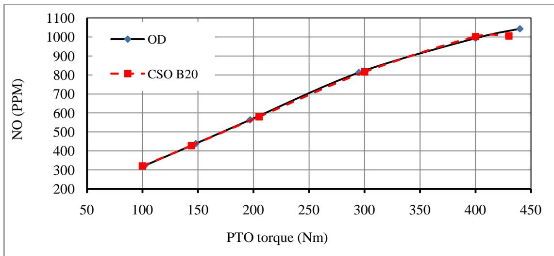
**Figure 9.** The relationship between PTO torques (Nm) and NO (PPM) for CD and CSO-B20
