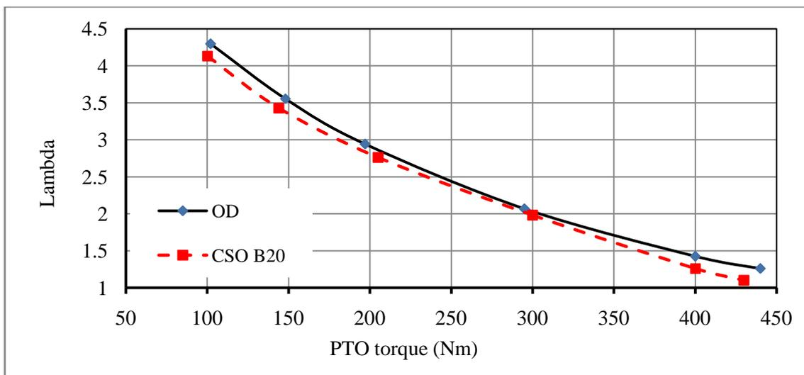
**Figure 11.** The relationship between PTO torques (Nm) and lambda ( $\lambda$ ) for CD and CSO-B20
