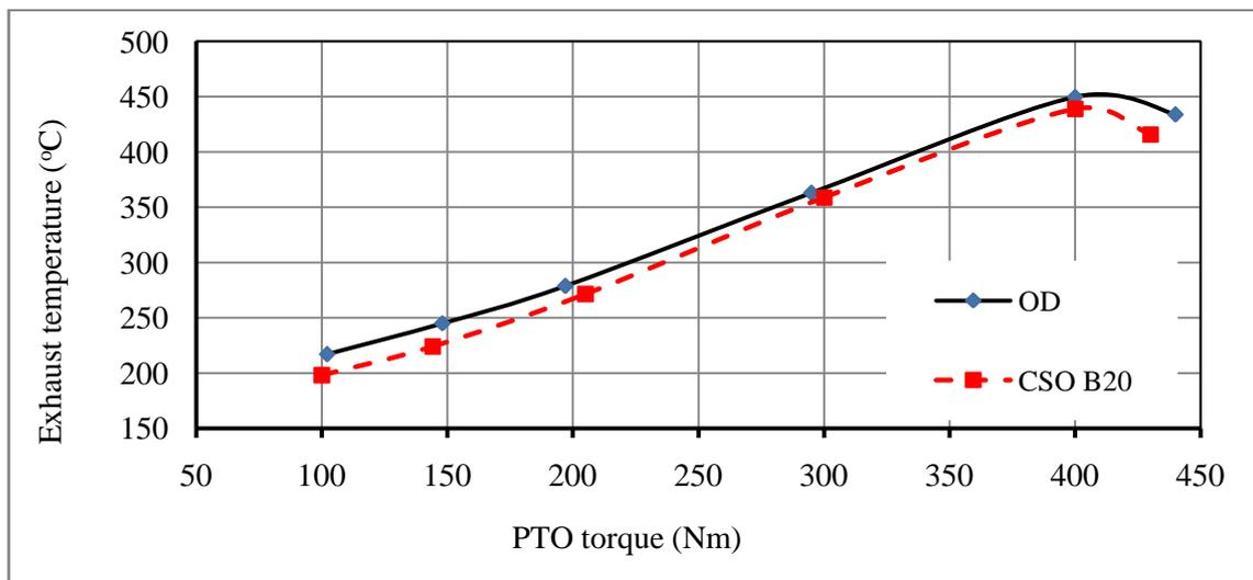
**Figure 6.** The relationship between PTO torques (Nm) and exhaust temperature (°C) for CD and CSO-B20
