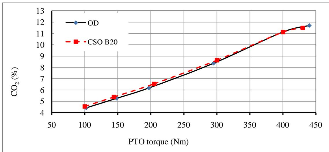
**Figure 8.** The relationship between PTO torques (Nm) and CO<sub>2</sub> (%) for CD and CSO-B20
