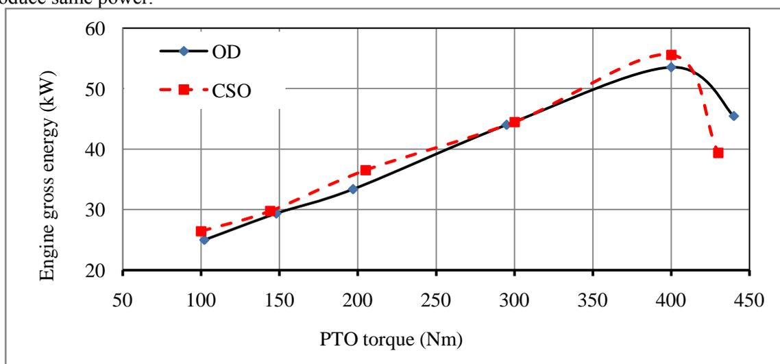
**Figure 3.** The relationship between PTO torques (Nm) and engine gross power (kW) for CD and CSO-B20
