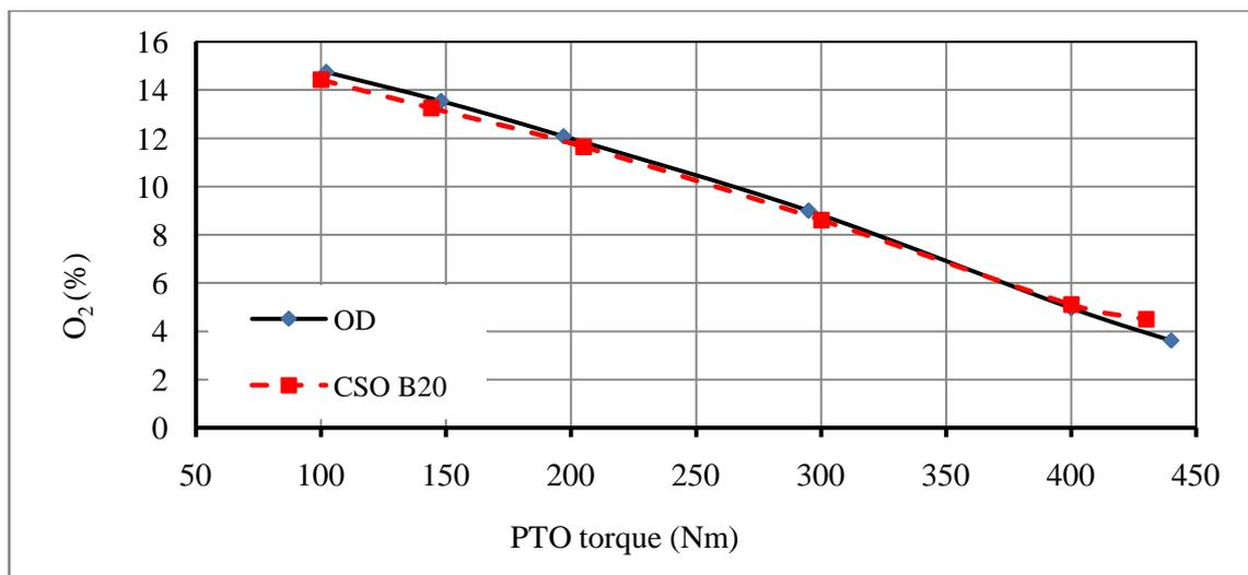
**Figure 10.** The relationship between PTO torques (Nm) and  $O_2$  (%) for CD and CSO-B20
