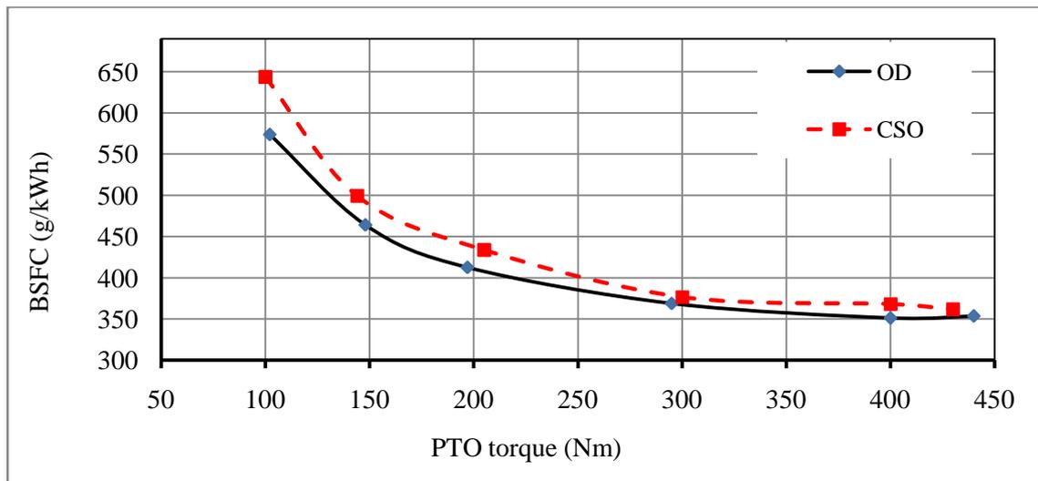
**Figure 4.** The relationship between PTO torques (Nm) and BCFC (g/kWh) for CD and CSO-B20
