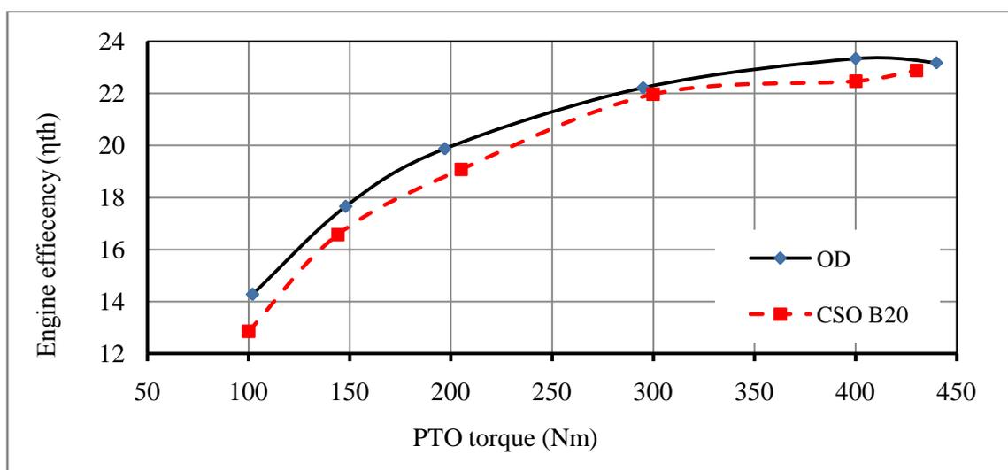
**Figure 5.** The relationship between PTO torques (Nm) and engine brake thermal efficiency ( $\eta_{th}$ ) for CD and CSO-B20
