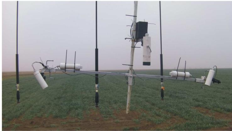
**Figure 3:** Three infrared thermometers on centre pivot irrigation in USDA-ARS at Bushland, Texas
