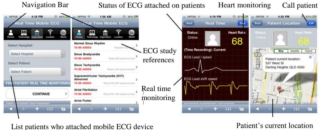
Figure 1. The mobile ECG decision support system in a smart phone device
