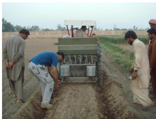
**Figure 4:** Field test of cotton seed dropping
