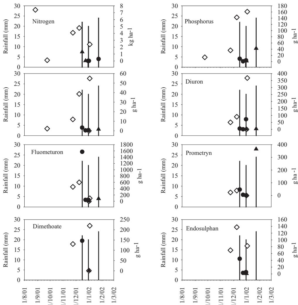
**Figure 5.** Total quantities of nutrients and pesticides in the runoff samples collected from each rainfall and irrigation event for furrow and subsurface irrigated sites in the first year (2001/2002). Dates are expressed in dd/mm/yy. Legend:  $\diamond$  = Furrow Irrigation,  $\bullet$  = Subsurface Drip Irrigation at 120% ETC,  $\blacktriangle$  = Subsurface Drip Irrigation at 90% ETC.
