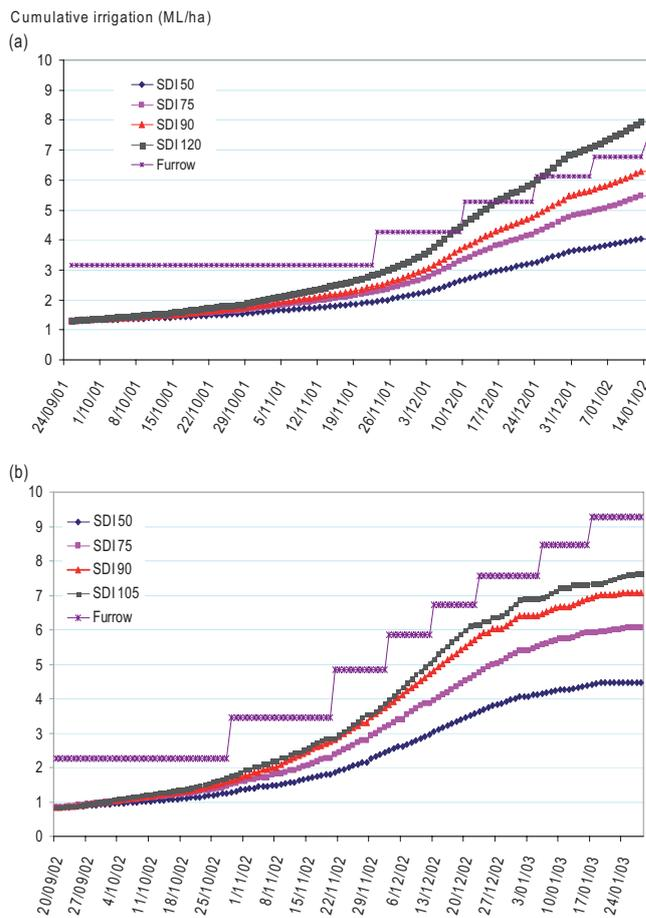
**Figure 2.** Cumulative applied water ( $\text{ML ha}^{-1}$ ) over the crop period for different irrigation treatments in year one (top) and year two (bottom). SDI: subsurface drip irrigation rate in percentage of crop evapotranspiration rate (see Sect. 2.2).
