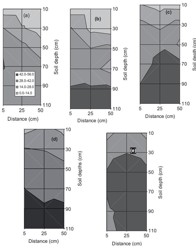
**Figure 3.** Soil moisture at different depths and lateral distances from the row at 74 days after seeding for different treatments (a: SDI50; b: SDI75; c: SDI90; d: SDI105 and e: FI) in the second year (measurements taken three hours after irrigation). Values are soil water depth mm 100 mm<sup>-1</sup> soil depth. SDI: subsurface drip irrigation rate in percentage of crop evapotranspiration rate (see Sect. 2.2). FI: furrow irrigation.
