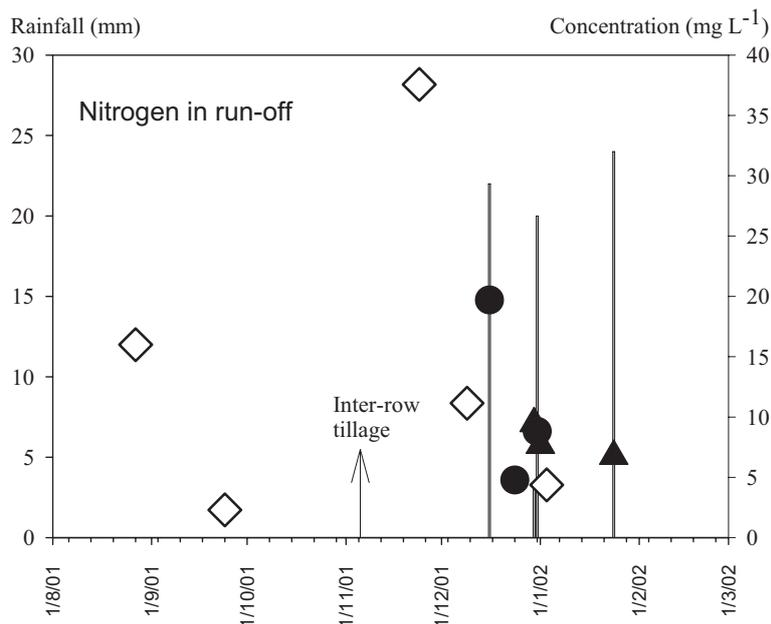
**Figure 4.** Nitrogen concentration in the different run-off events after irrigation and/or rainfall for cotton in the first year (2001/2002). Legend: ◇ = Furrow Irrigation; ● = Subsurface Drip Irrigation at 120% ETC; ▲ = Subsurface Drip Irrigation at 90% ETC.
