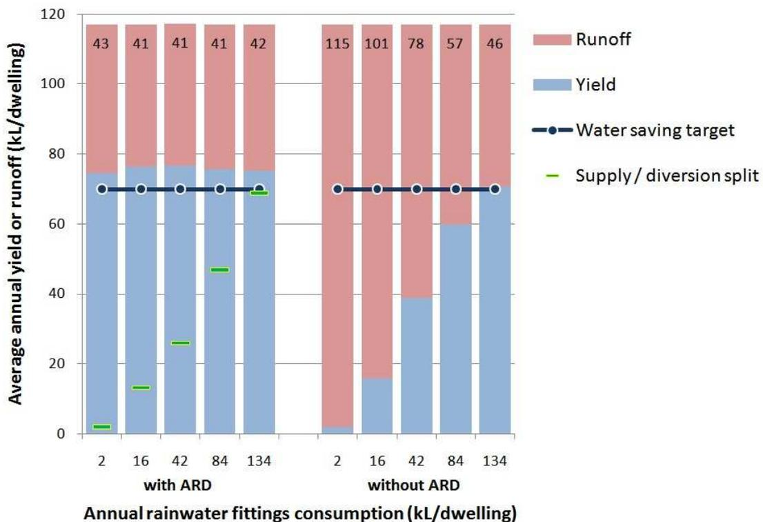
**Figure 3** Rainwater harvesting dual performance with and without ARD, for a connected roof area of 150 m<sup>2</sup>, in Brisbane and with performance by consumption scenario
