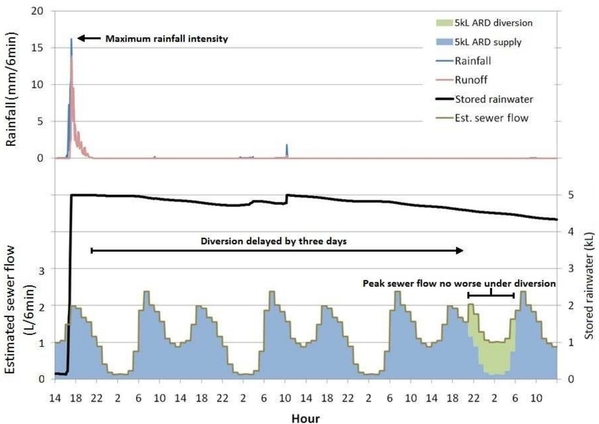
Figure 5 ARD system response to an excessive rainfall event for Brisbane
