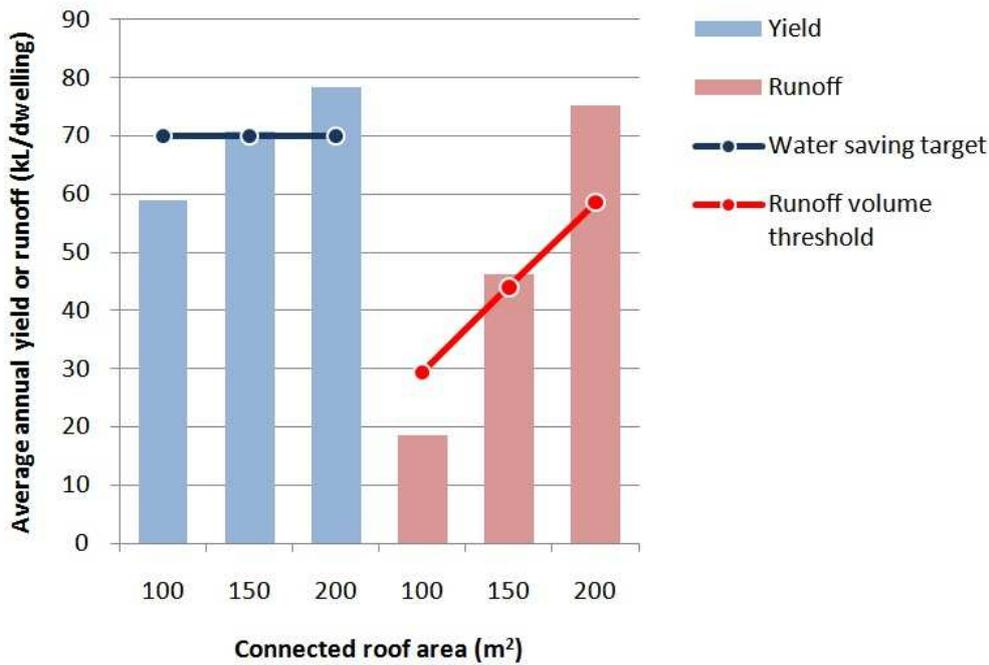
**Figure 2** Average annual yield and runoff from conventional rainwater harvesting, when supplying all non-potable fittings, for the average sized dwelling in Brisbane and with performance by connected roof area
