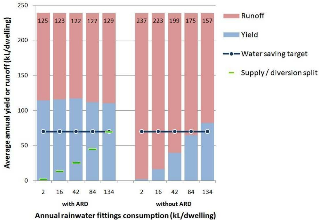
Figure 6 Rainwater harvesting dual performance with and without ARD, for a connected roof area of 150 m<sup>2</sup>, in Gold Coast and with performance by consumption scenario
