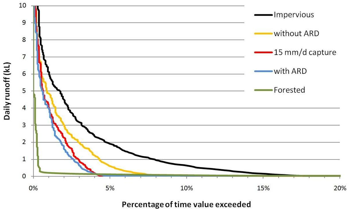
Figure 4 Flow duration curve for runoff events from 150 m<sup>2</sup> catchment under different conditions in Brisbane
