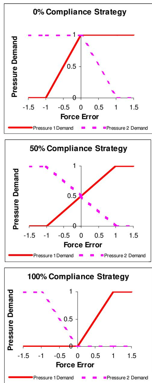
Fig. 2. Variable Compliance Strategy in a Pneumatic Cylinder
