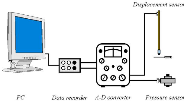
**Fig. 6: Data acquisition system**
