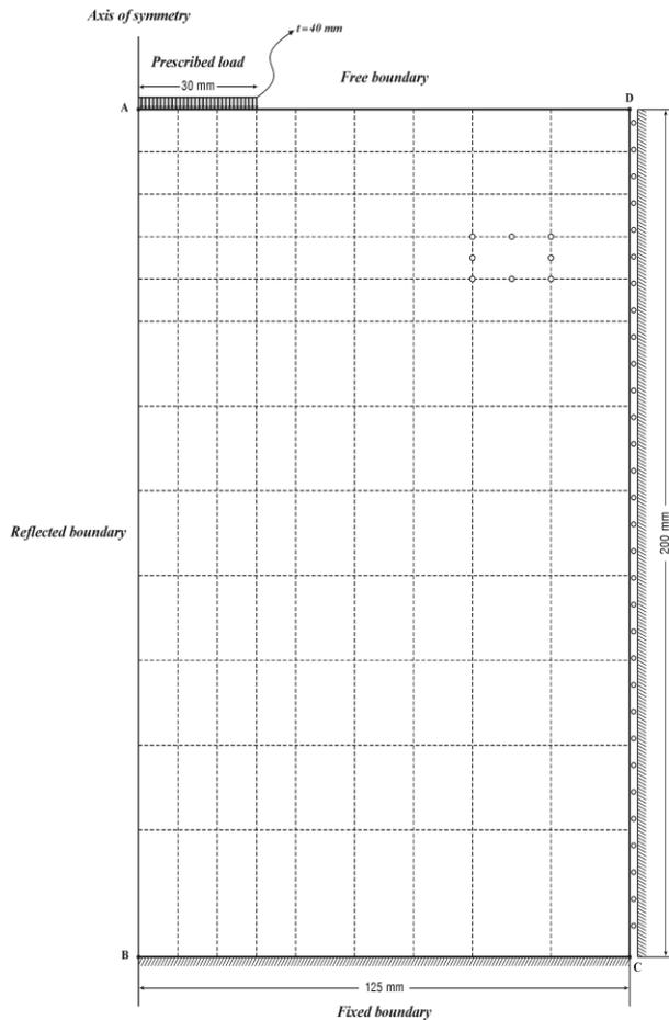
**Fig. 2: Two-dimensional FEM mesh of the soil-rectangular plate system**
