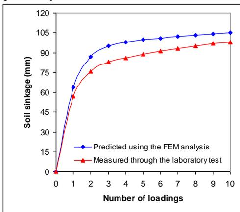
**Fig. 7: Soil sinkage values under the rectangular plate as related to number of loadings predicted using the FEM analysis in compared with those measured through the laboratory test**
