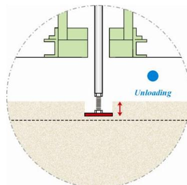
**Fig. 4: Unloading process**
