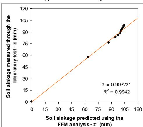
**Fig. 8: Soil sinkage values predicted using the FEM analysis and soil sinkage values measured through the laboratory test are plotted against each other and fitted with a linear equation with zero intercept**
