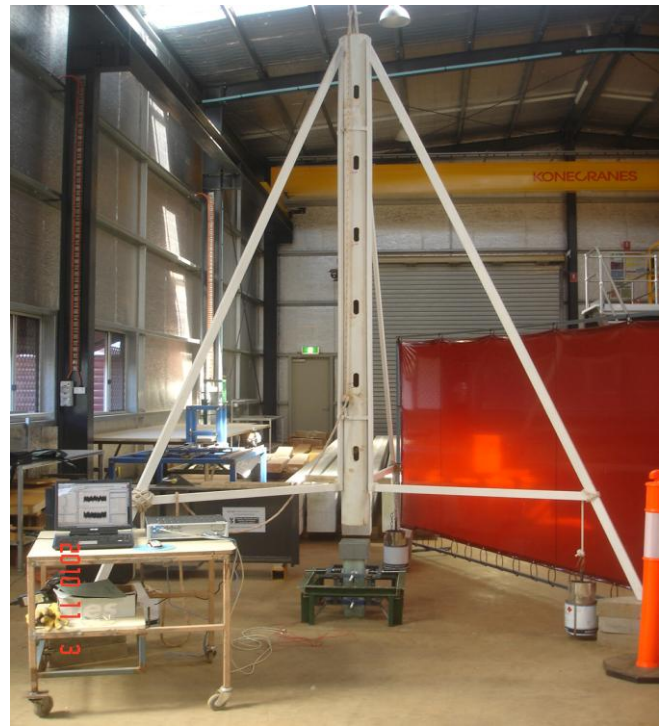
FIGURE 07: Testing set-up and drop impact test apparatus.
