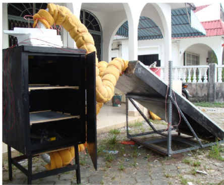
Fig. 1 Picture of indirect forced circulation solar drying thermal system.
