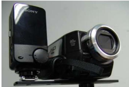
**Figure 2: Sony HDV (HC-5E) and Infrared Illuminator**
